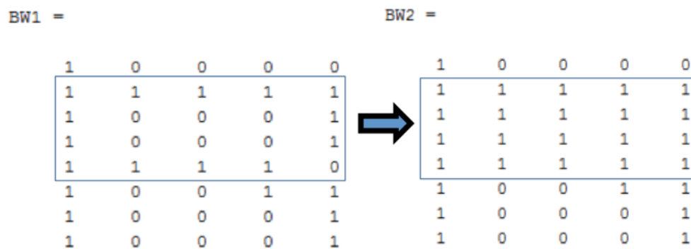
Figure 4.15. Filling all image binary holes to reduce noise (Binary Masking).
