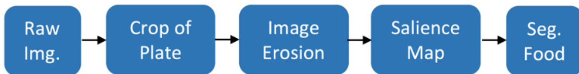
Figure 4.14. The segmentation algorithm flowchart.
