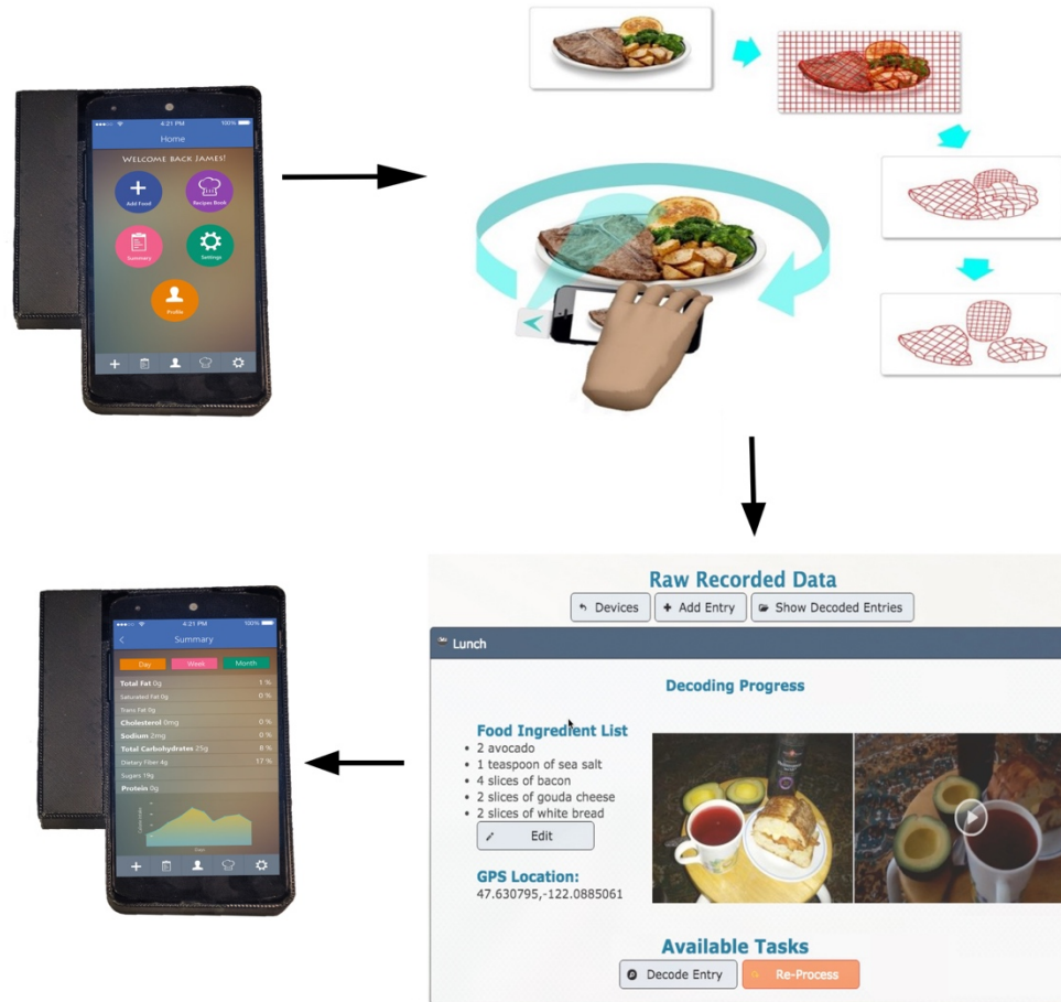
Figure 3.3. Digital Dietary Recording System (DDRS) overall system overview.
