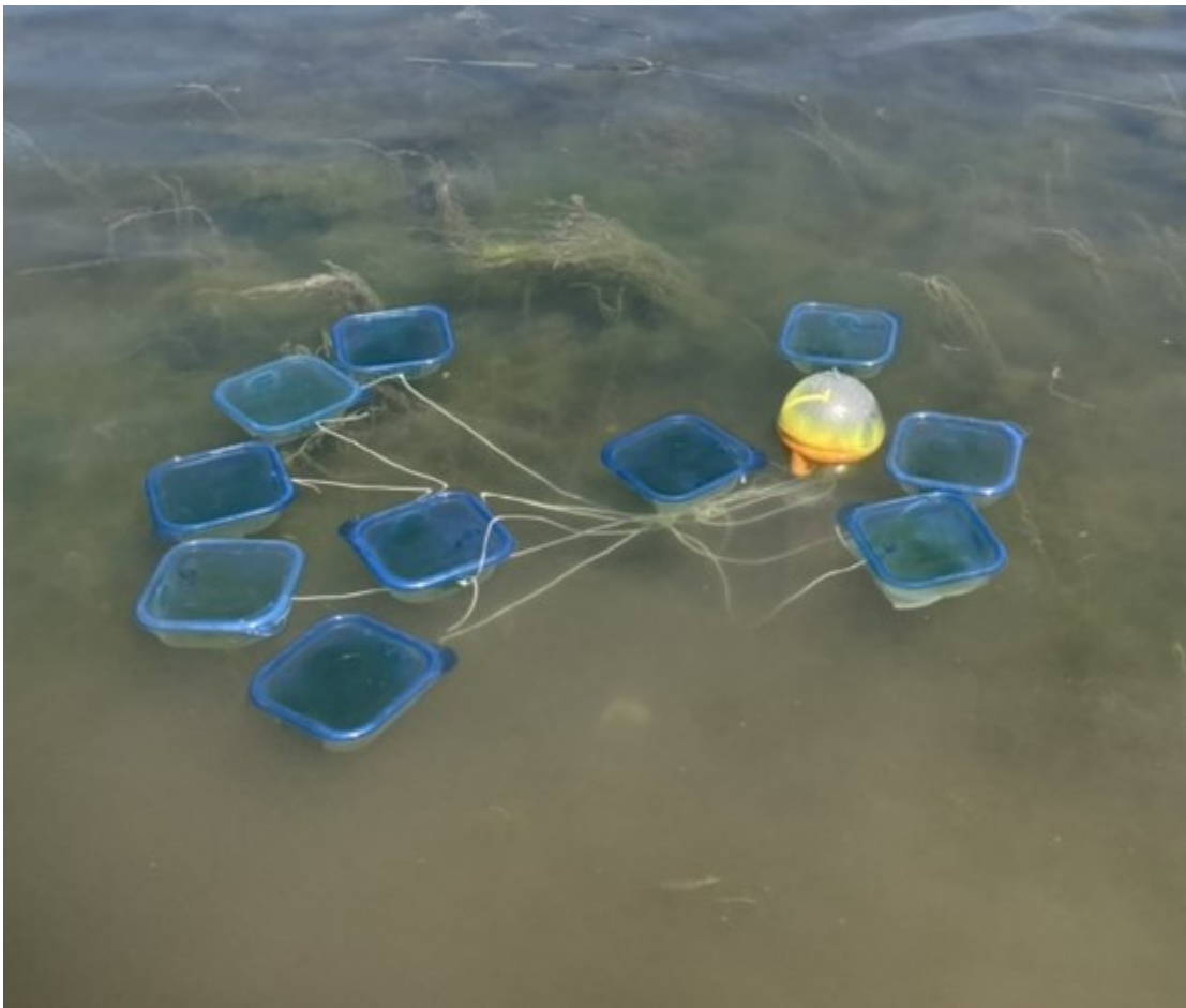
Figure 2: Field deployment setup, plastic containers each contain one egg mass. Buoy was hold in place with a brick.
