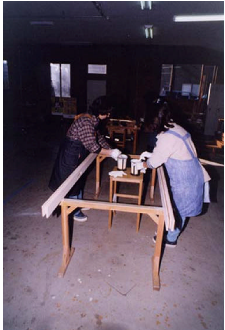
Figure 26. Workers manually apply a primer/sealer onto wooden window components.
