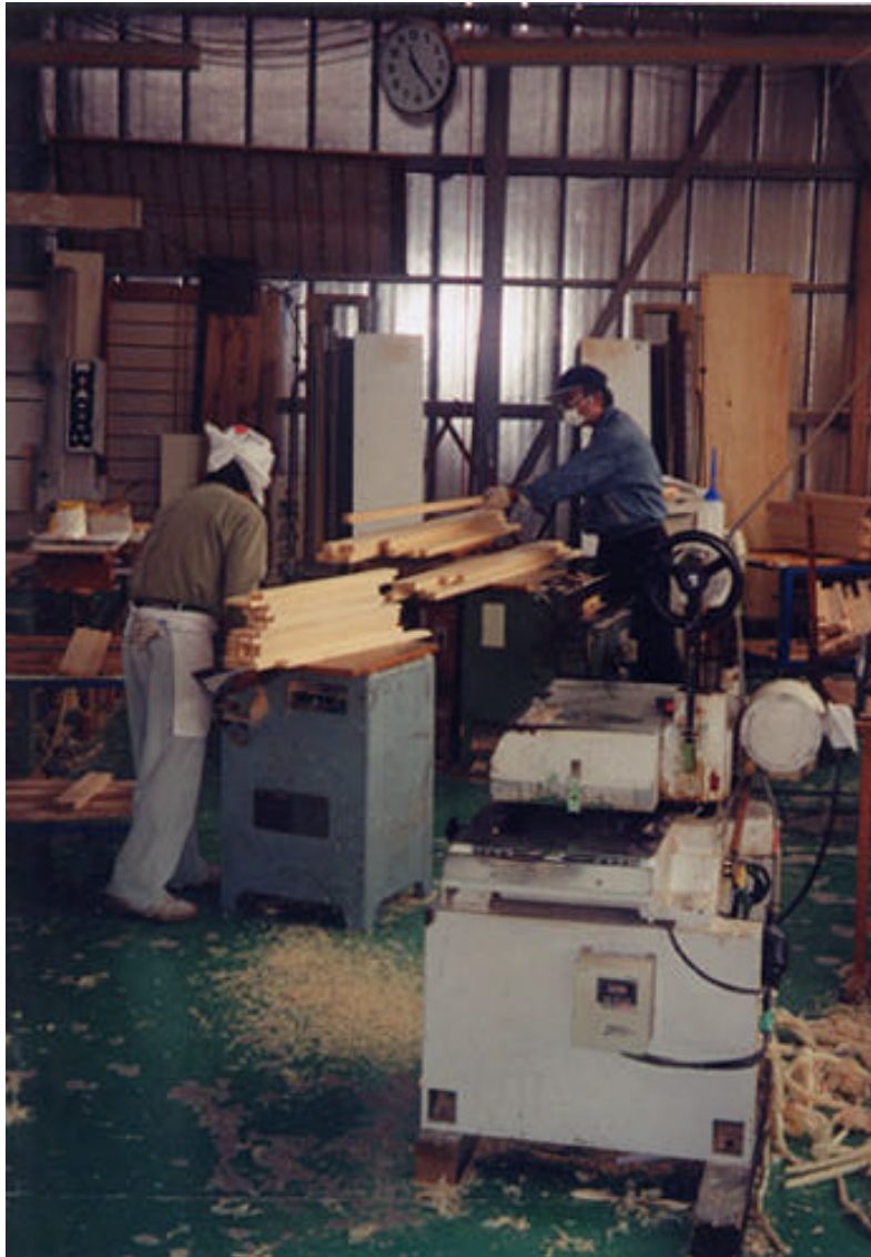
Figure 25. Window blanks are manually cut to size for assembly.
