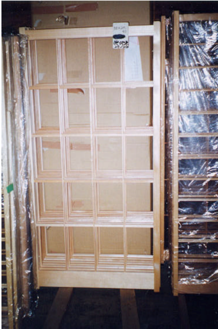
Figure 29. Shoji door ready for shipping. A paper face and back will be applied by another company prior to being installed.
