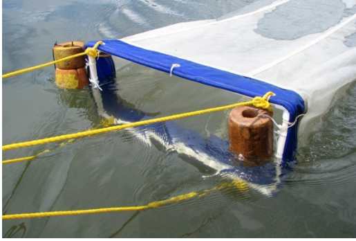
Small neuston net deployed during inundation.
