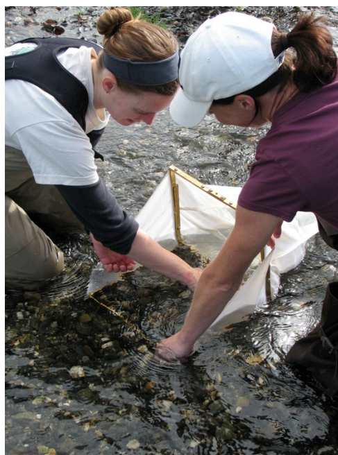
B-IBI sampling with Surber Sampler.
