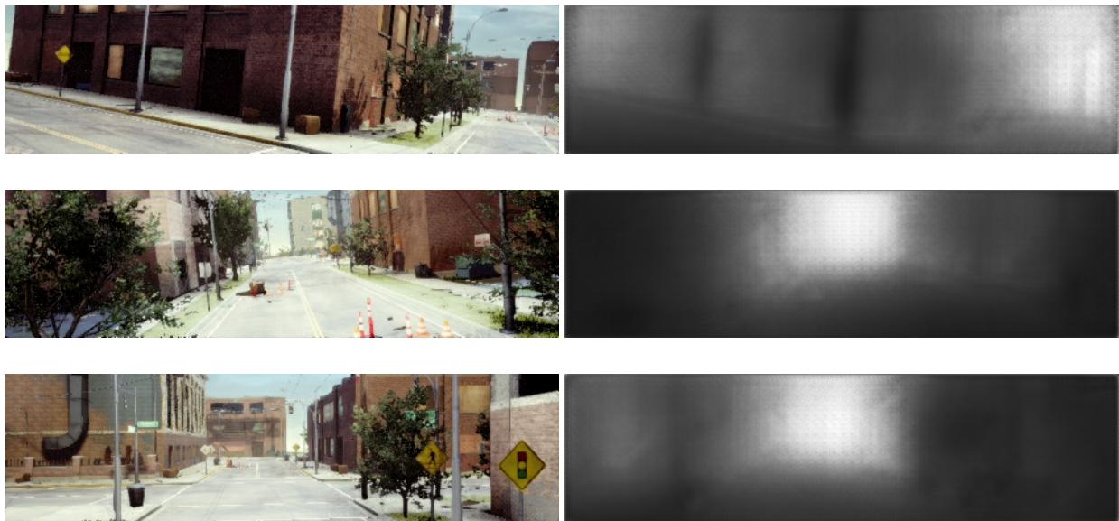
Figure 3.3: Sample images from the AirSim MAV dataset showing the RGB 480x128 resolution images in the left column and the learned depth image counterparts in the right column.
