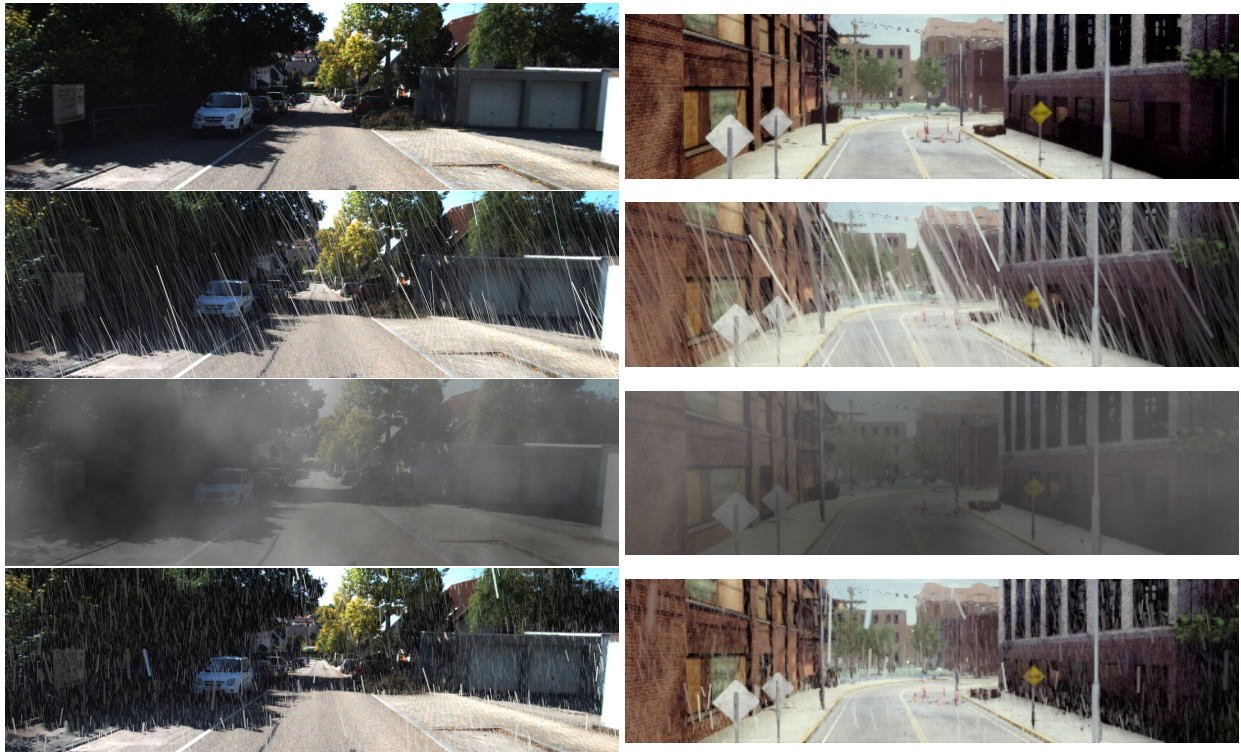
Figure 3.6: Sample images from the test trajectories with simulated harsh conditions. KITTI images are on the left with AirSim on the right. The top row is the unaltered image followed by the rain, fog, and snow conditions.
