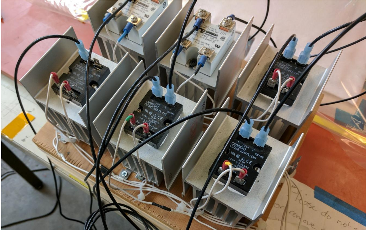
Fig. A4. Six of the twelve relays required to control six zones.
