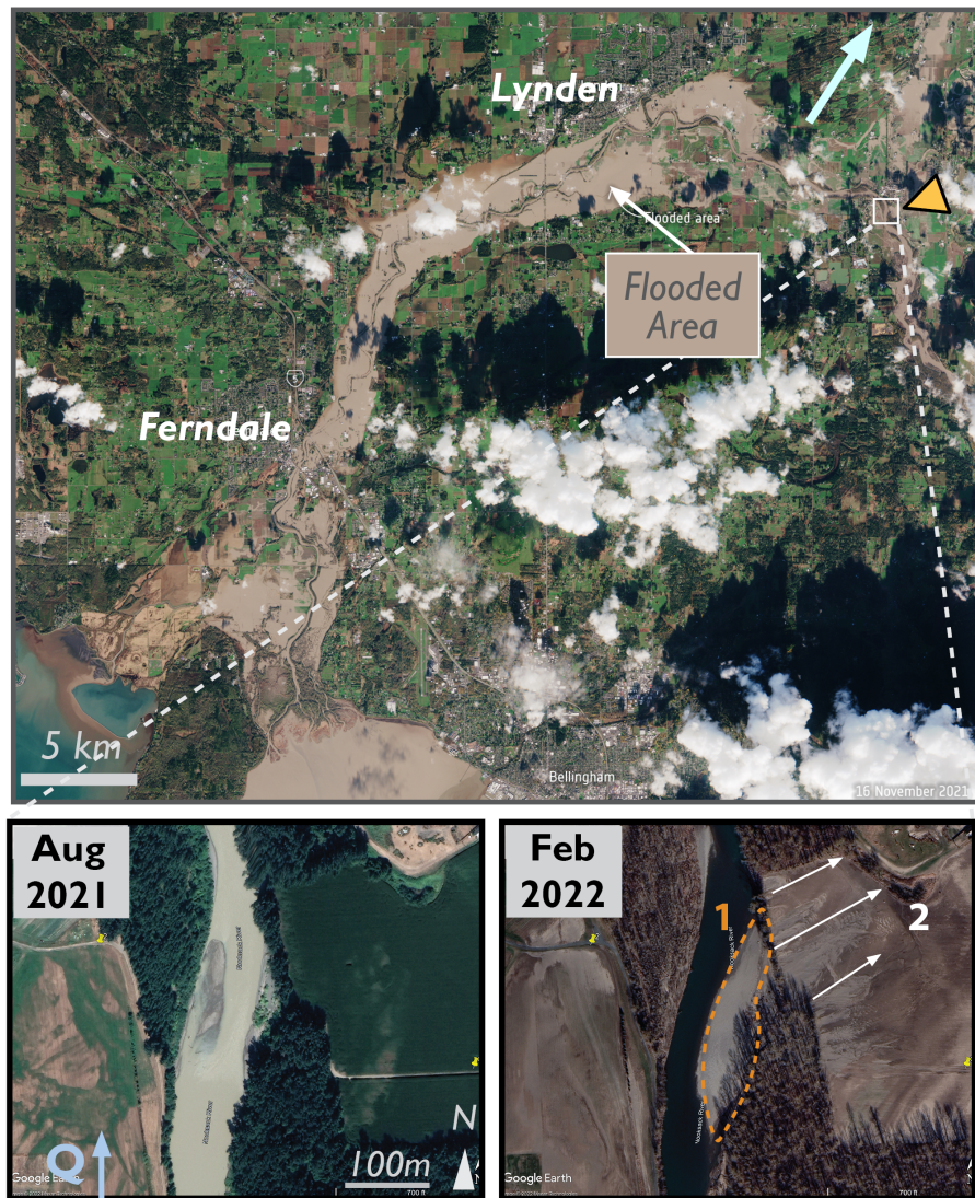
Figure 4.3: TOP: Satellite imagery on November 16 showing mud-colored flooded regions on the lower Nooksack and overflow north to Canada (imagery modified from Hansen et al. (2021)). BOTTOM: Nooksack channel at overflow site 3 months before (left) and after (right) November 2021 flood. Morphodynamic change occurred in the channel during the 2021 flood including deposition of (1) a river-right bar and (2) floodplain deposits reflecting the route of overbank flow. (Imagery from Google (2021); Maxar Technologies & Google (2022))
