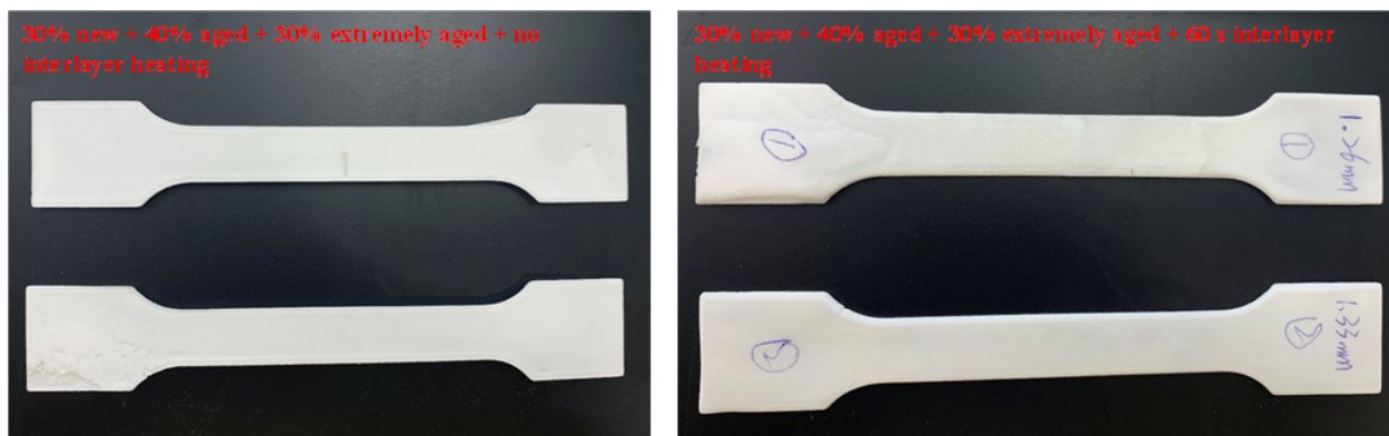
(g) Tensile bars with 30% new + 40% aged + 30% extremely aged powders
