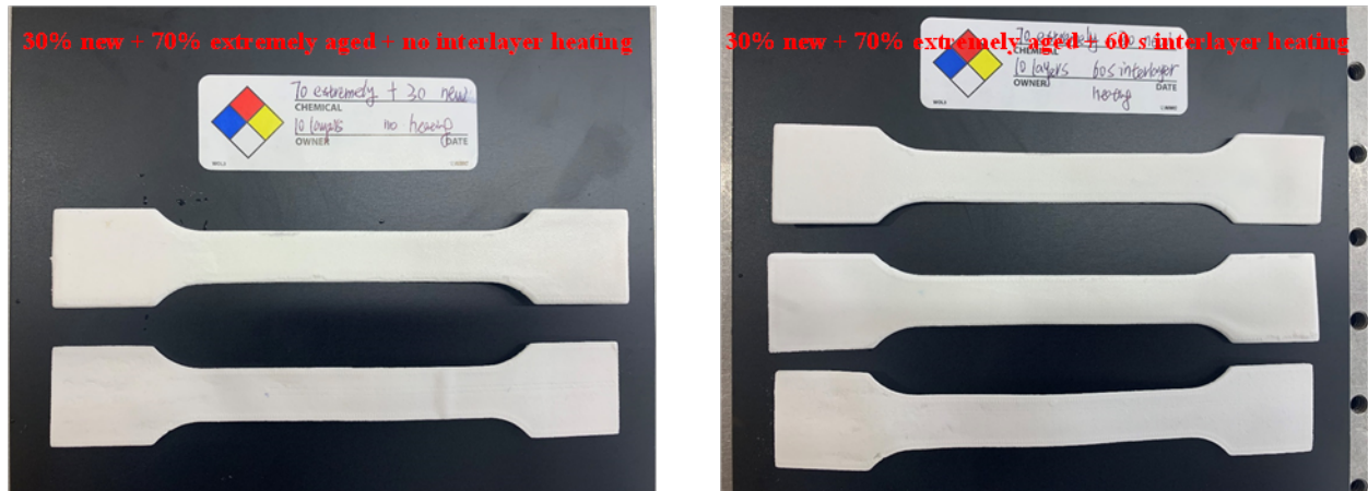
(d) Tensile bars with 70% extremely aged powders
