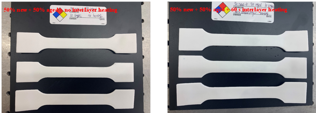
(a) Benchmark tensile bars with and without interlayer heating
