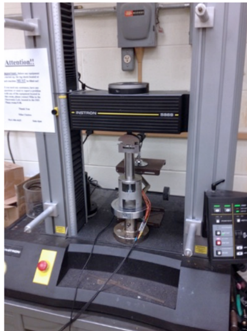
(b) Tensile test machine - Instron 5869
