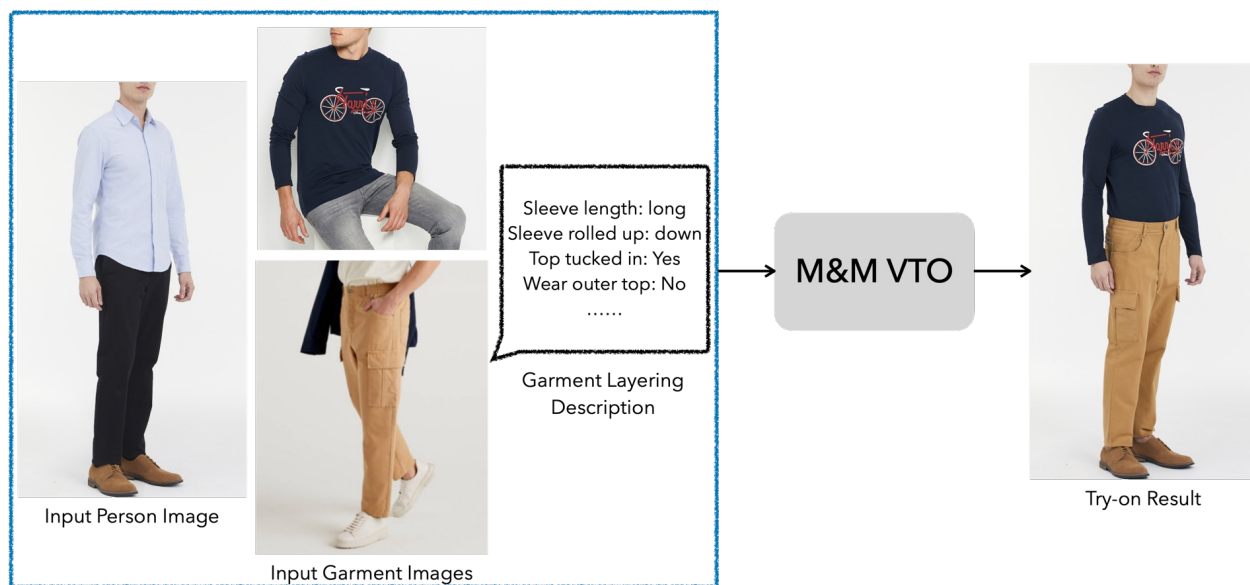
Figure 1.5: Task definition for M&M VTO. Given an image of upper body garment, an image of lower body garment, a text description of garment layout, and an image of a person, M&M VTO generates a visualization of how those garments (in the desired layout) would look like on the given person.
