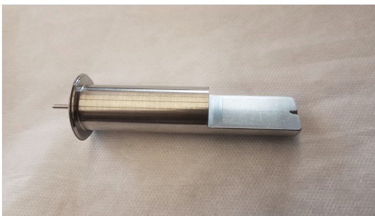
Figure 6.6: Photo of the stainless steel ruler used for the CMOS camera image calibration. A 1.5 \times 3 cm grid pitched at 500 \mu\text{m} is laser-etched onto the flat face.
