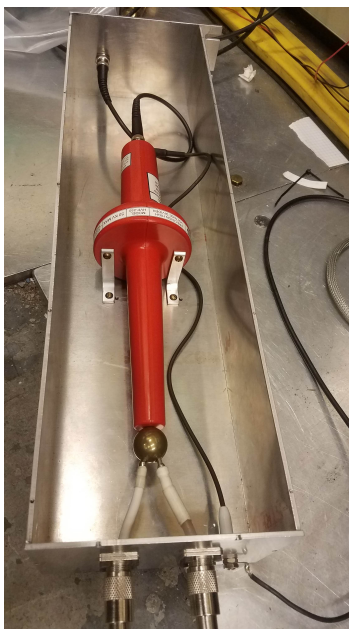
Figure 3.6: The CPS HV probe used to calibrate the HV divider readings.
