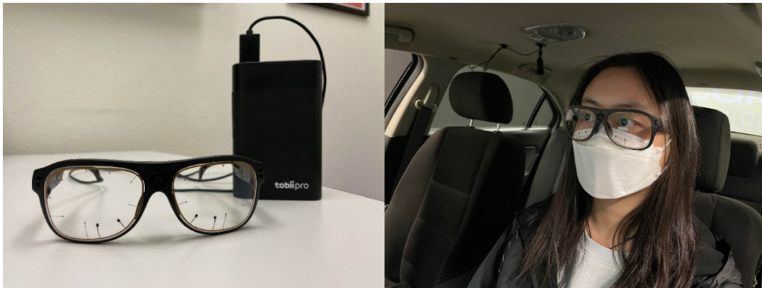
Figure 5.3 OSU Eye Tracking. Left: Tobii Pro Glasses 3 with Recording Unit. Right: Tobii Pro Glasses 3 Worn by a Researcher.
