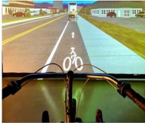
Figure 5.1 OSU Bicycling Simulator from the participant's perspective
