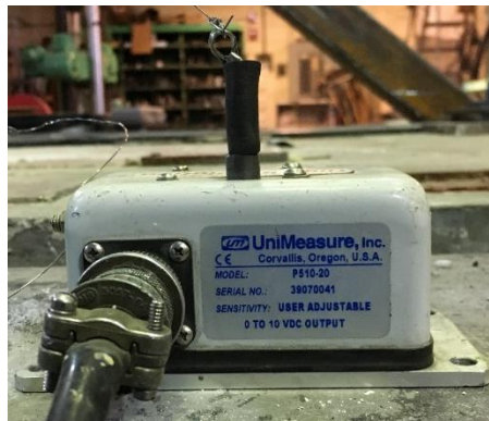
Appendix Figure H.5. UniMeasure ® string potentiometer.
