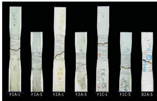
Figure 7.2. Ductal ® UHPC direct tension cracking field.
