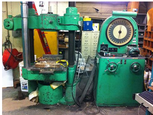
Appendix Figure H.2 300-kip Baldwin testing machine.
