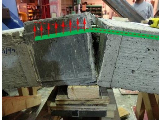
Figure 7.8. Upward force distribution from bent reinforcement.
