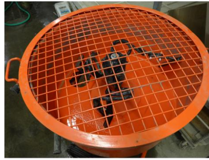
Appendix Figure H.1. Pan mixer used to mix UHPC.
