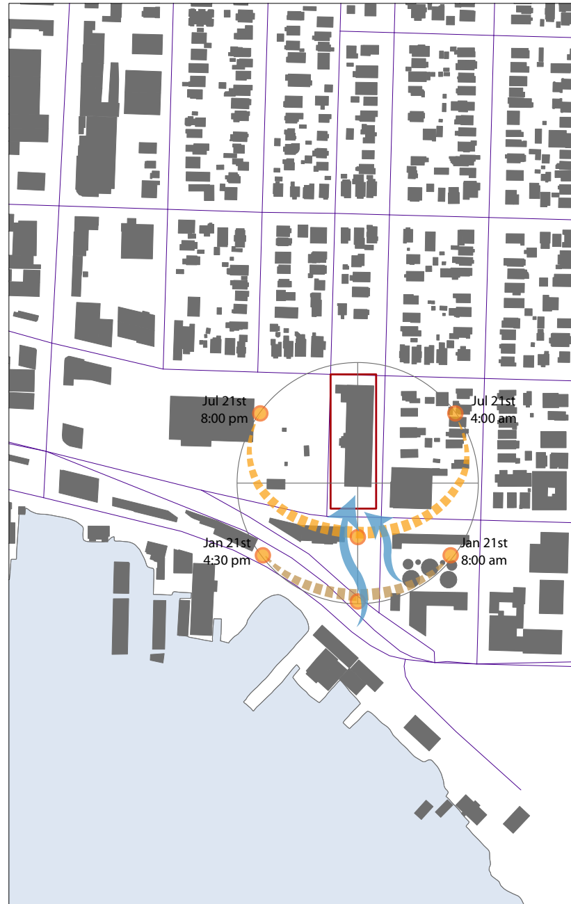
Fig. 3.7 Solar and wind analysis for the site
