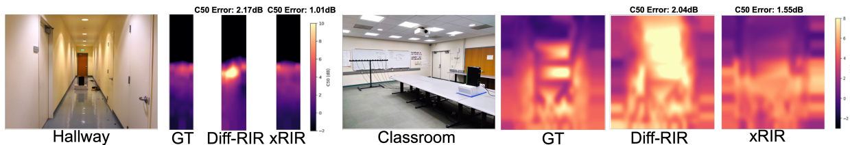
Figure 8.5: Qualitative Comparisons of Acoustic Map Predictions in Two Real Environments: a Hallway and a Classroom. We visualize the acoustics maps by computing the C50 metric at dense locations in the entire room and compare with the ground-truth acoustic map. xRIR achieves C50 distributions that better matches the ground-truth. (Figure from [XL6])
