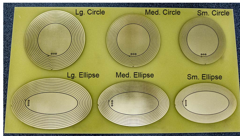
Figure 5.19: PCB antennas designed by model optimization.
