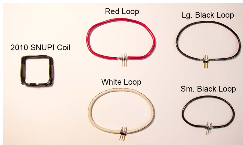
Figure 5.17: Wire-wound antennas evaluated. This includes the antenna design used on the original SNUPI node (square, black loop), and four single turn antennas with varied area, wire thickness, and solid-core vs. stranded wire.
