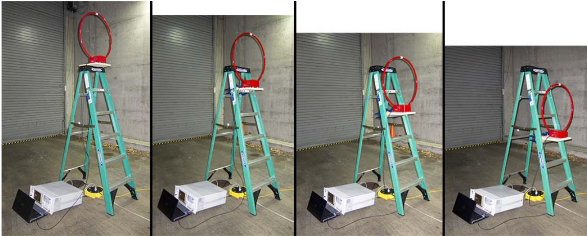
Figure 3.11: Various heights of receiving antenna used to avoid nulls in the field pattern.
