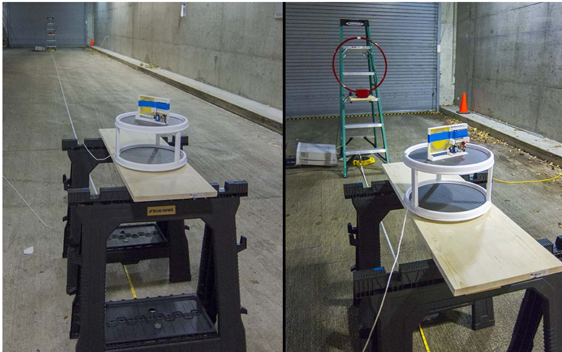
Figure 3.10: Experimental setup for field strength measurements. The transmitter and receiver were placed 20 m apart ( left ) for 13.56 MHz, and 3 m apart ( right ) for 27.00 MHz. The FCC recommends 30 m of separation at 13.56 MHz, but the basement used for measurement was not large enough to support measurements at more than 20 m of separation.
