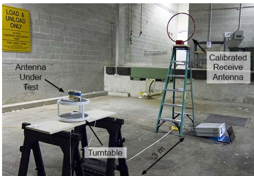
Figure 5.21: Picture of antenna radiated power measurement.
