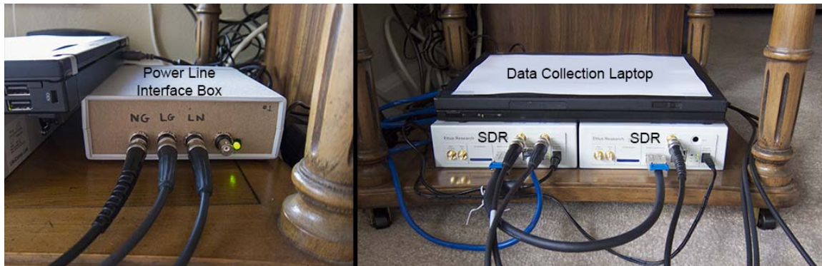
Figure 3.1: Hardware used for background noise data collection, including a custom made power line interface, two software defined radios (SDR), and a data collection laptop.
