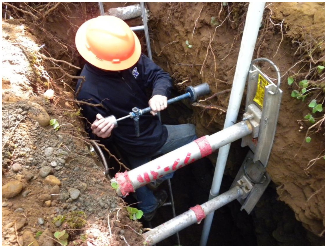
Figure 2.2. Bulk density sampling at Oil City Road, south of Forks, WA. Careful shoring was used to ensure safety while working in the soil pits.
