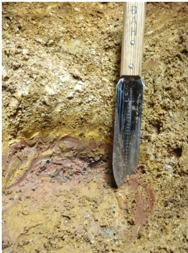
Figure 2.8. Close-up of transitions between 2Bt2, 3Btm1, and 3Btm2 horizons at the bottom of the soil profile at Silver Creek. Tick marks on soil knife are 5 mm apart.
