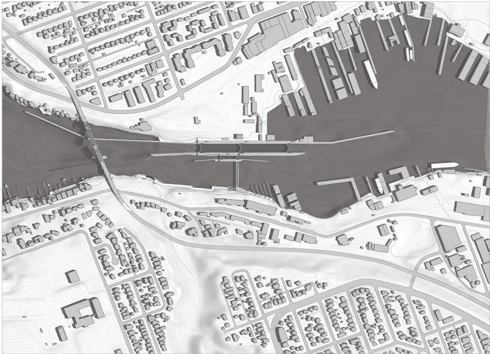
Figure 4.1: This plan of the Locks and context represents historical bathymetry contours with solid lines, current contours and bathymetry contours with dashed lines, and the navigation channel with larger dashed lines.
