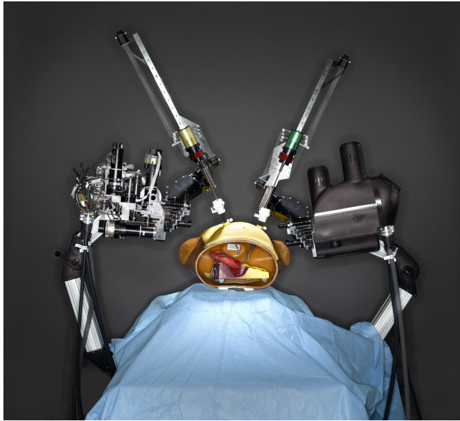
Figure 1.1: The RAVEN I surgical research robot developed at the University of Washington BioRobotics lab.
