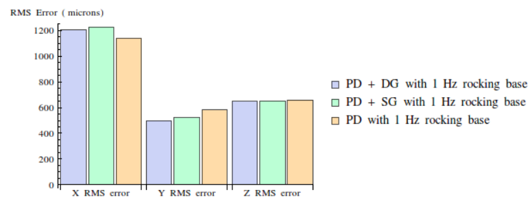
Figure 5.11: RMS of X, Y, and Z position error for the three controllers during autonomous trajectory with rocking base.
