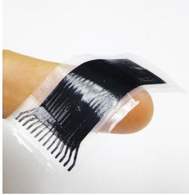
Figure 58. Completed DES laminate after removal from glass substrate.
