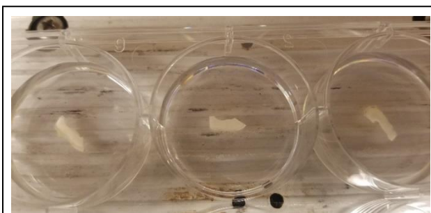
Figure 8: Dentin specimens in a 6-well plate on an automated shaker. From left to right, the well plates contain the specimens in the remineralization solution at pH's of 6.8, 7.0, and 7.4 respectively.
