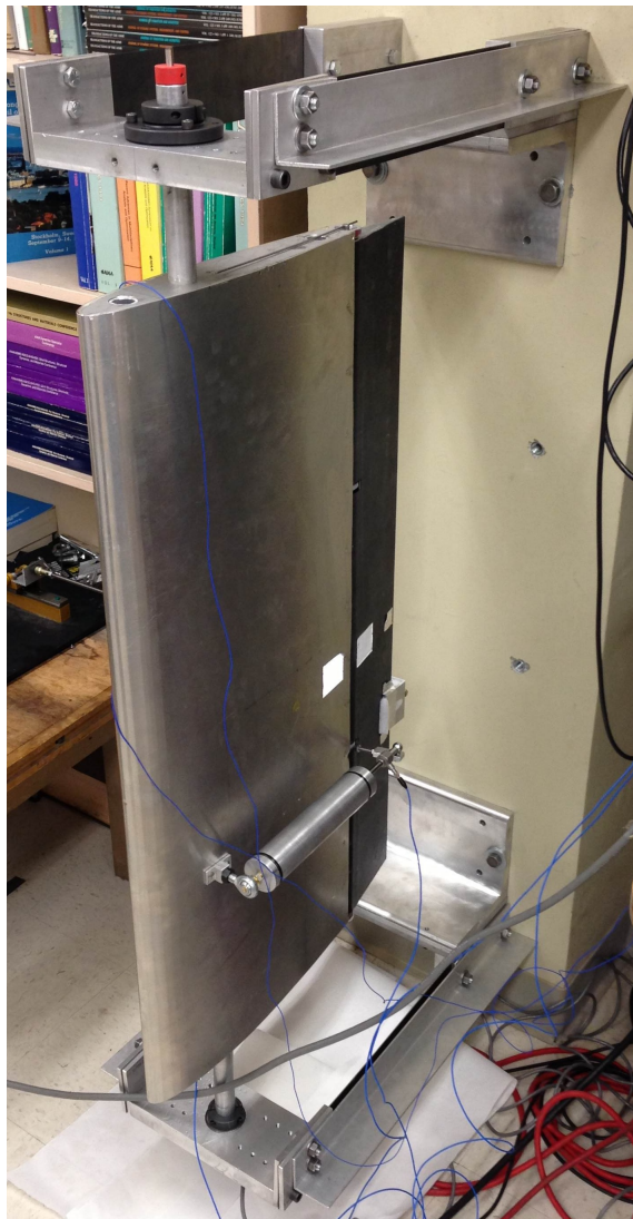
Figure 3.4: University of Washington aeroelastic system mounted in lab [8].
