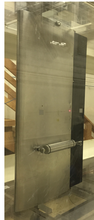
(b) View of the model in the test section with dampers attached
