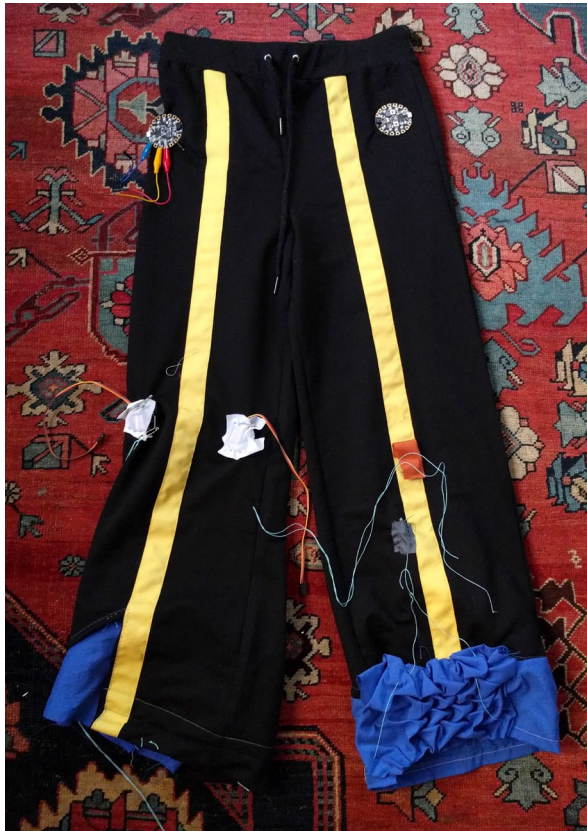
Figure 17a. Basting stitches and power mesh to secure servos.
