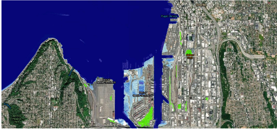
Figure 11. Close up of a NOAA sea level rise viewer climate change map of south Seattle with 5-foot mean higher high waters (MHHW) projections in light blue and bright green..
