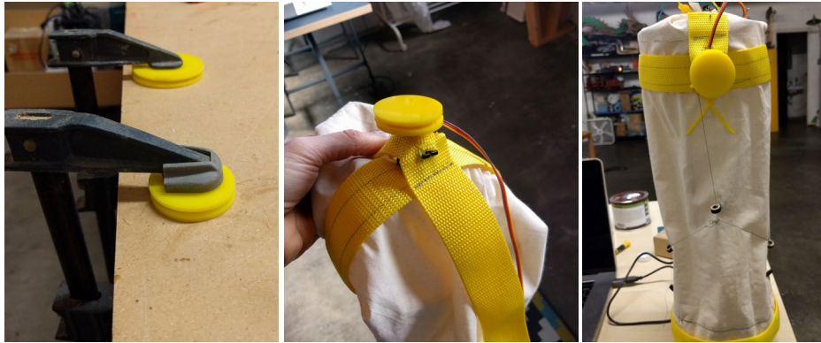
Figure 19. The motor was placed at the very top of the model leg since I visualized it being right below a cyclist's knee joint. I attached the servo motor at the narrower part of the base, which is a weaker way to attach it so I strapped it on with nylon webbing and attempted to make a small x-shaped support structure. I also used the nylon webbing to strap the servo to the pants and add structure to the top and bottom of the pants. I sewed on a series of laser cut loops to guide string being pulled and later modified the string with butterfly clips to investigate how adding 'stopping' mechanisms could make the pull of the spool bunch up the pants in a more evenly distributed way.
