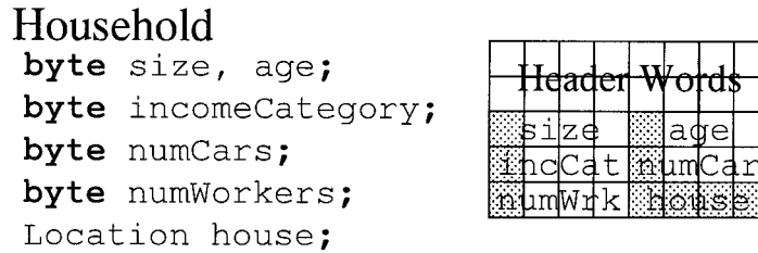
Figure 2.1: Fields and memory layout of a typical Household object, showing how much memory may be lost due to per-instance overhead. In the figure on the right, shaded boxes are those required to store the fields as declared in the Household definition, with empty boxes showing overhead. One small box represents one byte of memory.
