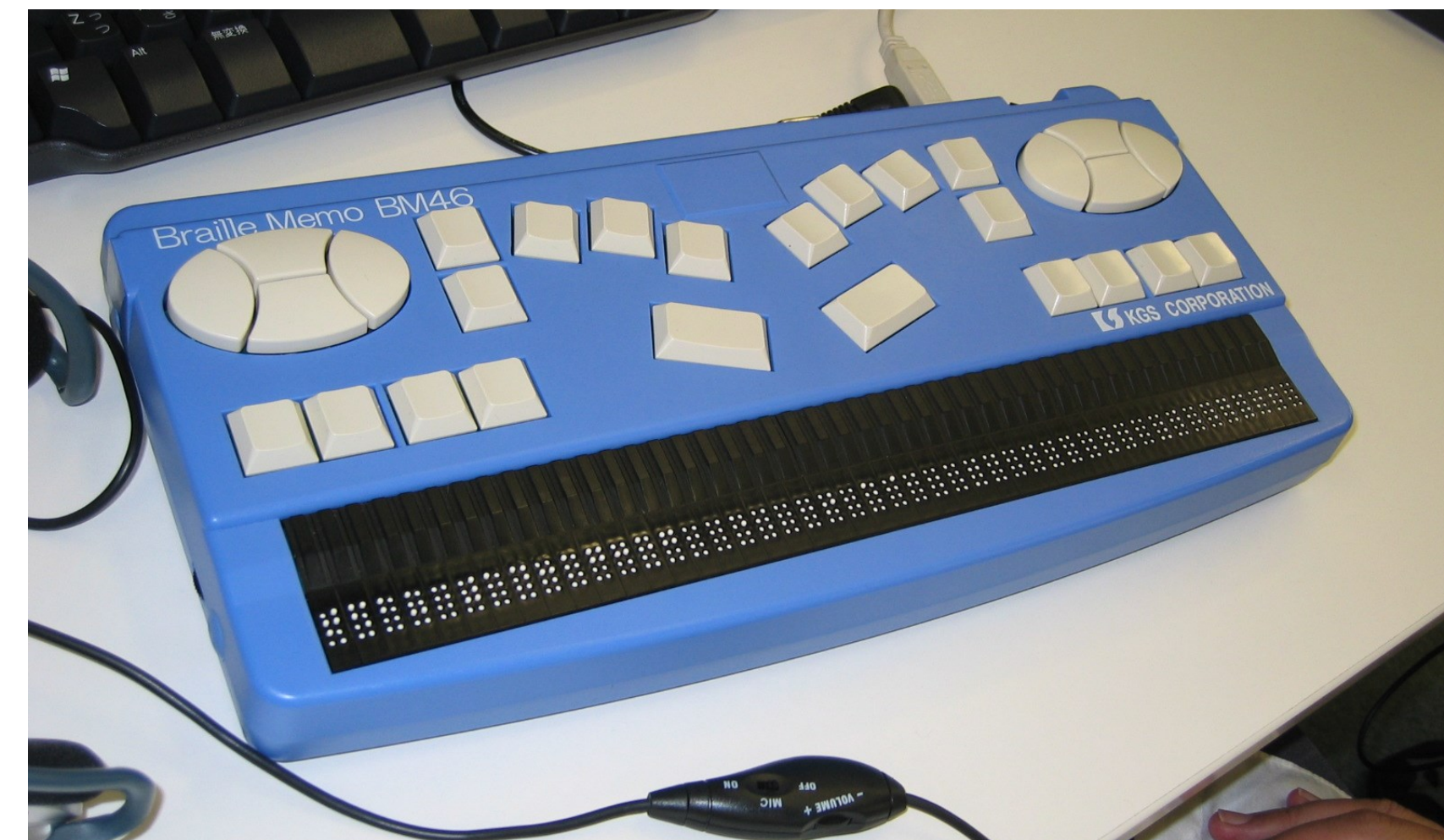
This braille keyboard adaptor allows for the use of braille transcription with a computer setup. When a human being produces braille, that is called braille transcription. A computer producing braille is known as braille translation.
