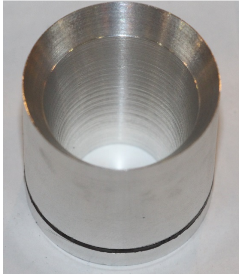
Figure 3.12: Example projectile used for LGG-capture plate experiments.
