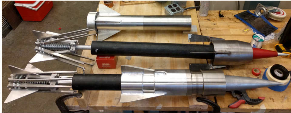
Figure 5.1: Mock up of drop articles. From top to bottom: passively deployed hexcell ejecta brake article with steel-tipped penetrator, passively deployed Kevlar brake article with steel penetrator, timer-deployed Kevlar ejecta brake article with steel-tipped penetrator.
