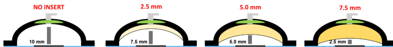
Figure 4.4. Diagram indicating different dome volumes tested. Red text indicates thickness at the center of the insert. Black text and gray bar indicate size of void from the center of the dome.
