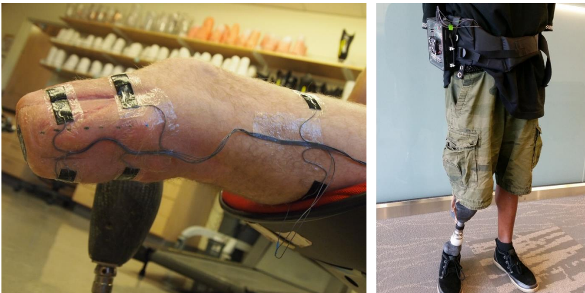
Figure 2.3. Portable bioimpedance analysis system. Bioimpedance electrodes placed on a residual limb (left) and a transtibial prosthesis user wearing a portable bioimpedance device on a waist belt. From [62].
