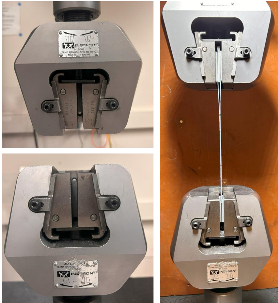
Figure 3.8 Load frame fixtures, (left) and specimen inserted inside fixture (right).
