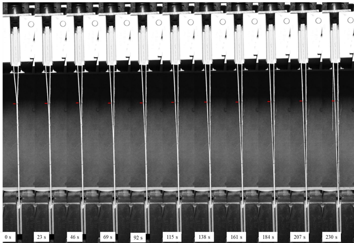
Figure 4.5 Laminate-A_Sample-7_4p8 specimen crack propagation with snaps at every 23s. The red mark indicates the initial crack length.
