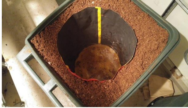
Figure 11: 96 Gallon Ice Target Lined With Pykrete
