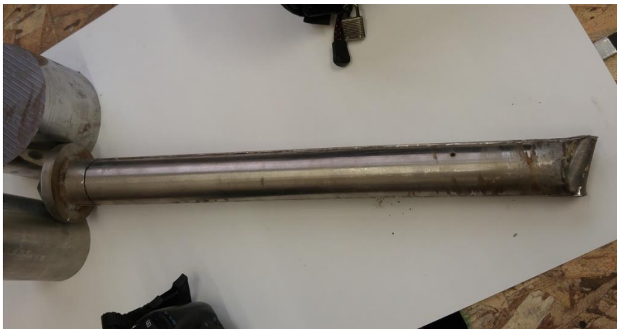
Figure 4: Successfully Ejected SRC from System with Oversized Ejection Chamber [1]
