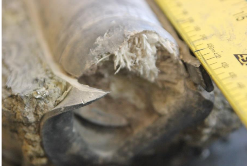
Figure 3: Close Up of Close Fitting Ejection Chamber Buckling with Impinged SRC [1]
