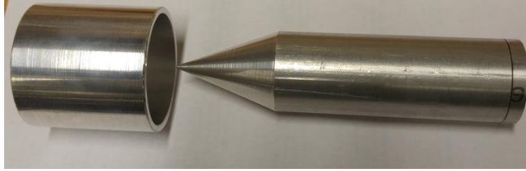
Figure 14: Two Projectile System for Accelerometer Deposition
