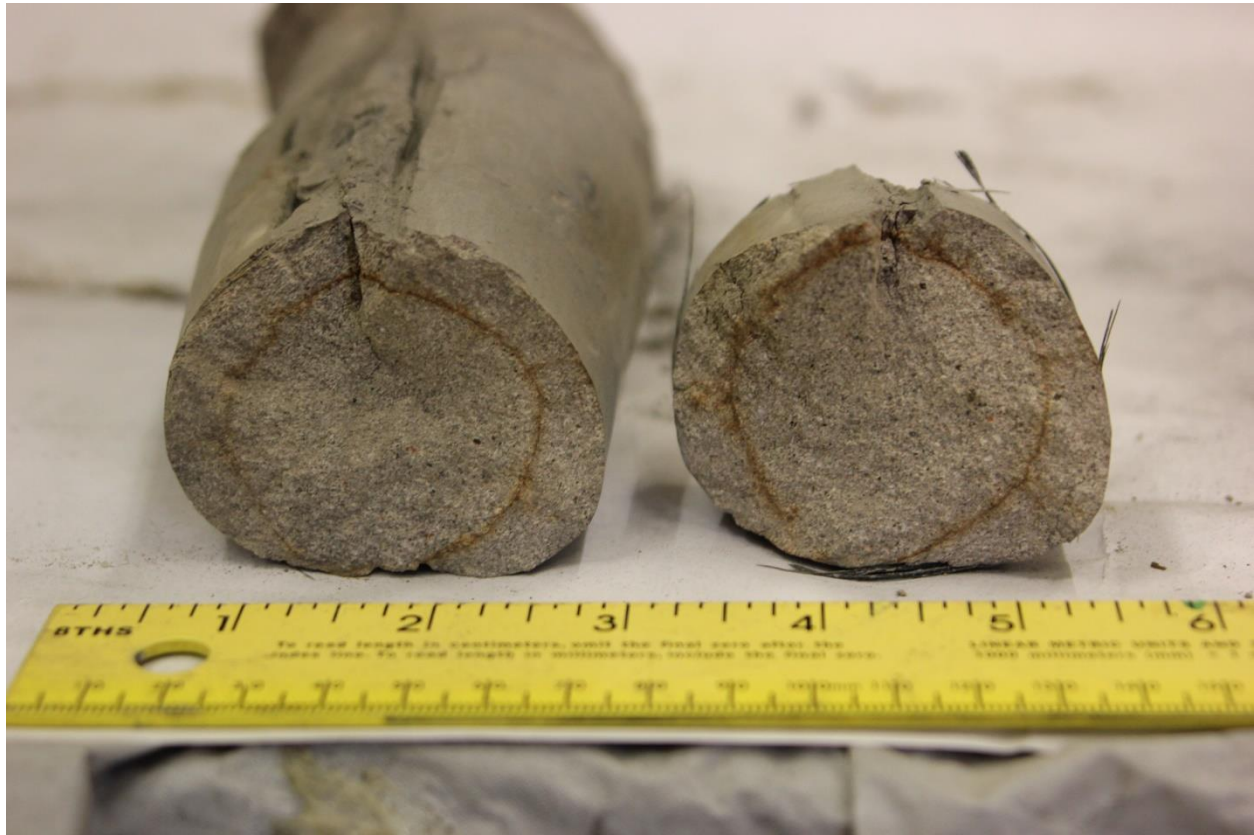
Figure 2: Center Bore and Side Port SRC Sample with Concentric Ring Possibly Caused by Boundary Effects [1]
