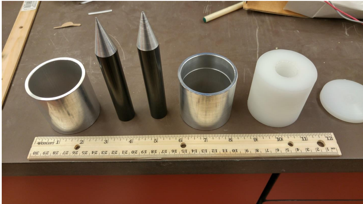
Figure 13: Low Pressure Air Gun Projectiles and Obturators
