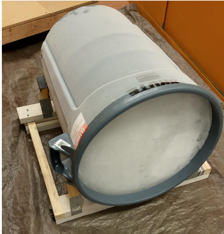
Figure 10: 30 Gallon Ice Target and Cradle
