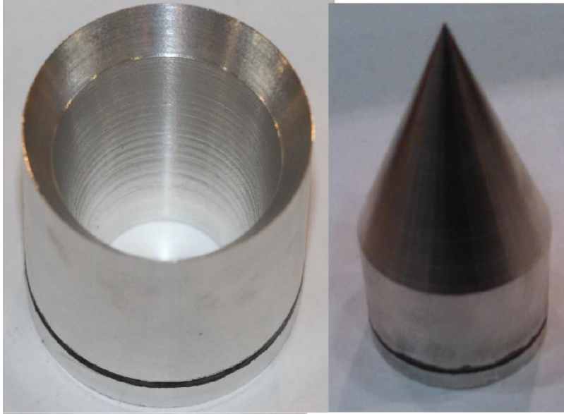
Figure 16: Cylindrical and Conical Projectiles for High Pressure Gas Gun
