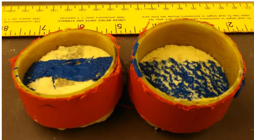
Figure 17: Kevlar and Fiberglass Projectiles Showing Differing Impact Energy from Tape Damage
