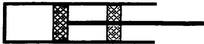
Figure 9-2: A cylinder closed by a piston. Students are asked what motion of the piston will result in positive work on the gas.
