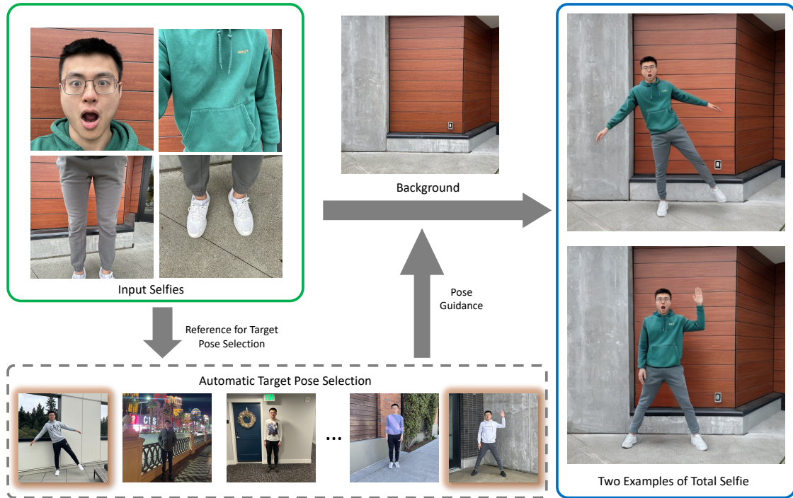
Figure 3.1: We generate full-body selfies of you (right), from self-captured images of your face and body (top left) and background. You can choose any target pose from a reference photo — we auto-select a set of good candidates from your photo collection (bottom).
