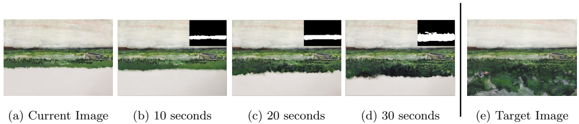
Figure 6.9: Ablation of time interval. (a) and (e) show the current and target image, respectively. (b) to (d) show the predicted next images and their masks (inset) given different time intervals. As the time interval increases, the size of the predicted mask expands, leading to more extensive updates on the canvas. Image courtesy Cleveland Museum of Art.
