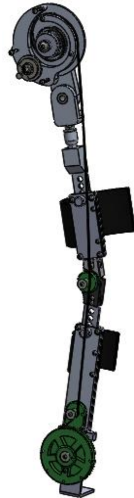
Figure 2-5: A unilateral assembly of PlayGait showcasing the spiral torsion spring in the hip assembly (top) connected to an exotendon wrapping anteriorly around the hip and knee pulleys and wrapping posteriorly around the ankle pulley.
