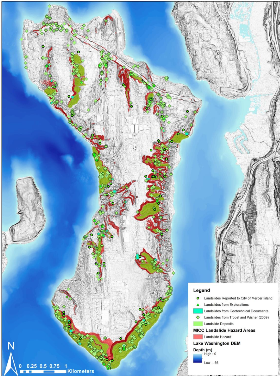
Figure 15. All identified, reported, and mapped landslides overlaid on the MICC landslide hazard map. 57% of reported and identified landslides fall within MICC landslide hazard areas.
