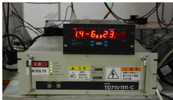
(d) Turbo-pump controller and Televac vacuum monitoring system.
