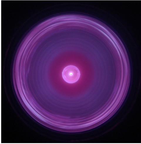
Figure 3.4: Uniform RMF discharge from an ELF-like, single cathode source located on-axis.
