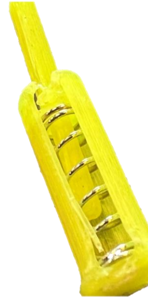
Figure 17. Iteration two print of Pin and Pin Body assembled with spring.
