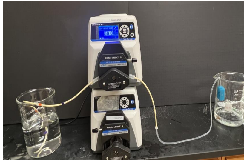
Figure 27. The Simulated Use characterization test set up for the final design. The PDMS tubing extending from the Backpack housing connects to the peristaltic pump via connections to additional tubing.
