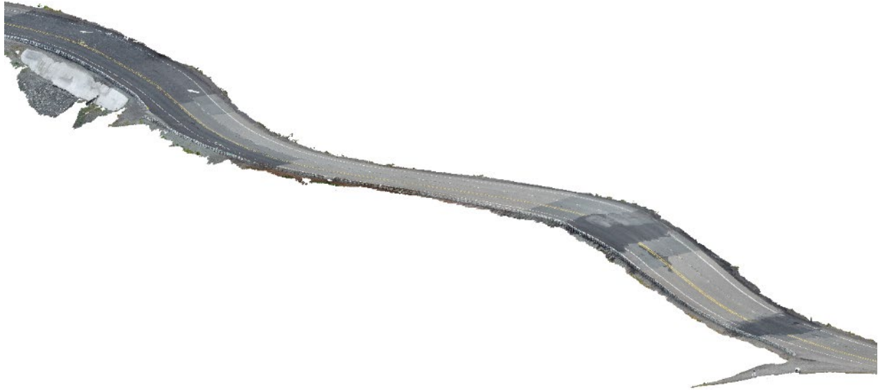
Figure 2.4. UAS-SfM dense point cloud data representation of the highway
