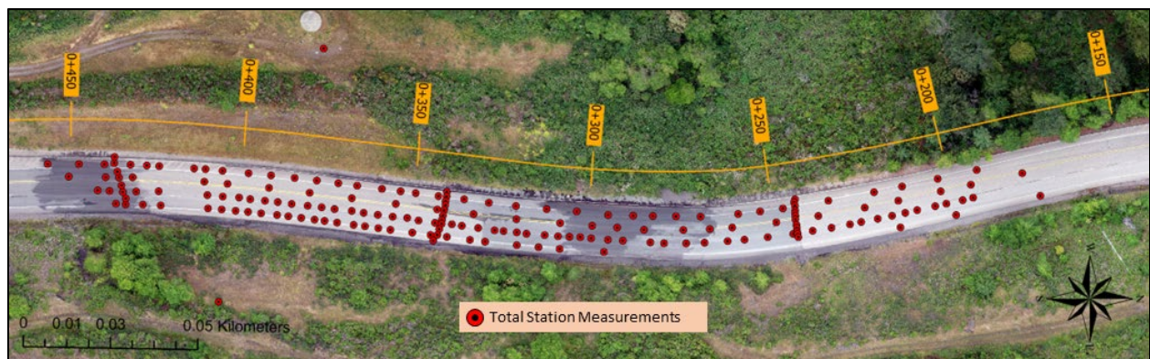
Figure 2.2. The check points on the road surface surveyed by the total station.
