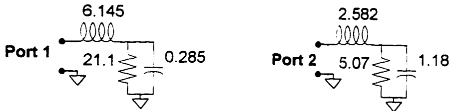
FIGURE 27. Uncoupled impedances looking into the transformer.
