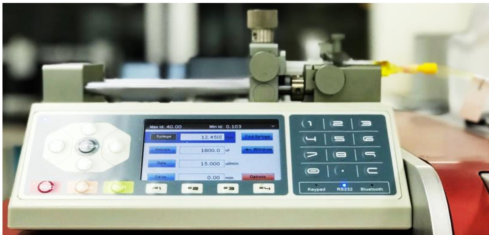
Figure 14 Syringe pump used to dispense perovskite ink
