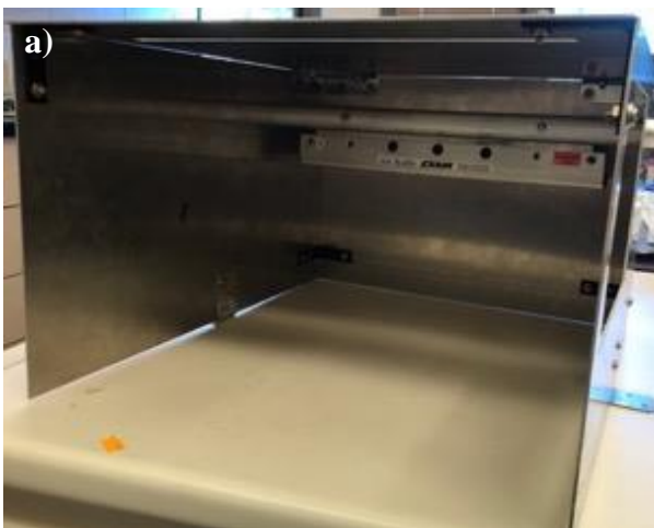
Figure 18 Picture of large area chamber in operation and with an air-knife a)Distance from the coating head to the air-knife b)Distance from the top of the air-knife to the bed
