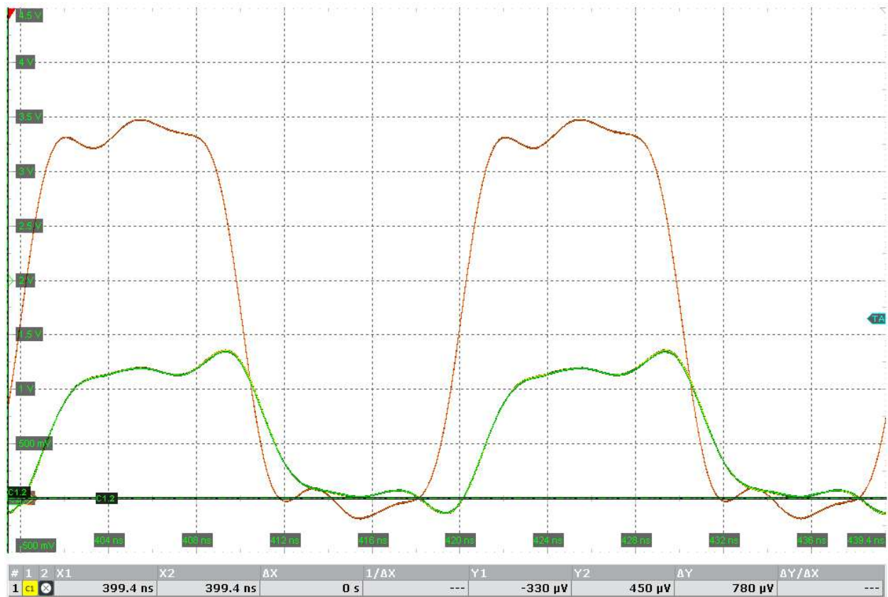
Figure 4.16. 50 MHz clock pulse direct from generator (orange) and on microstrip port 2 (yellow) and port 3 (green)
