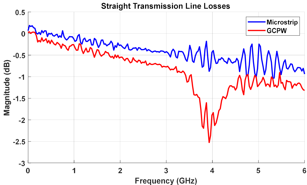
Figure 2.10. Loss for microstrip and GCPW straight transmission line
