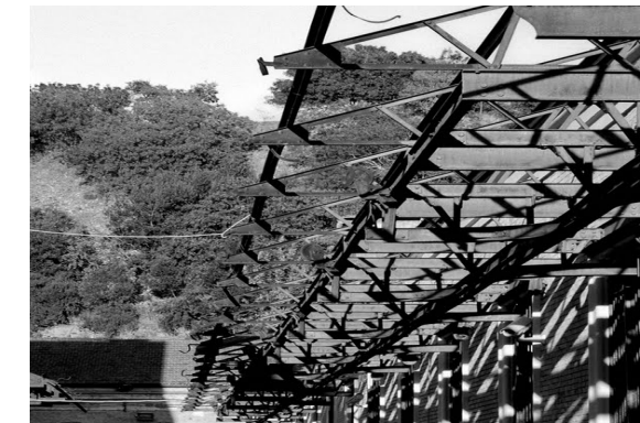
Figure98: Overhead rail system used to transport slaughtered livestock carcasses from one building to another in the Mattatoio.
