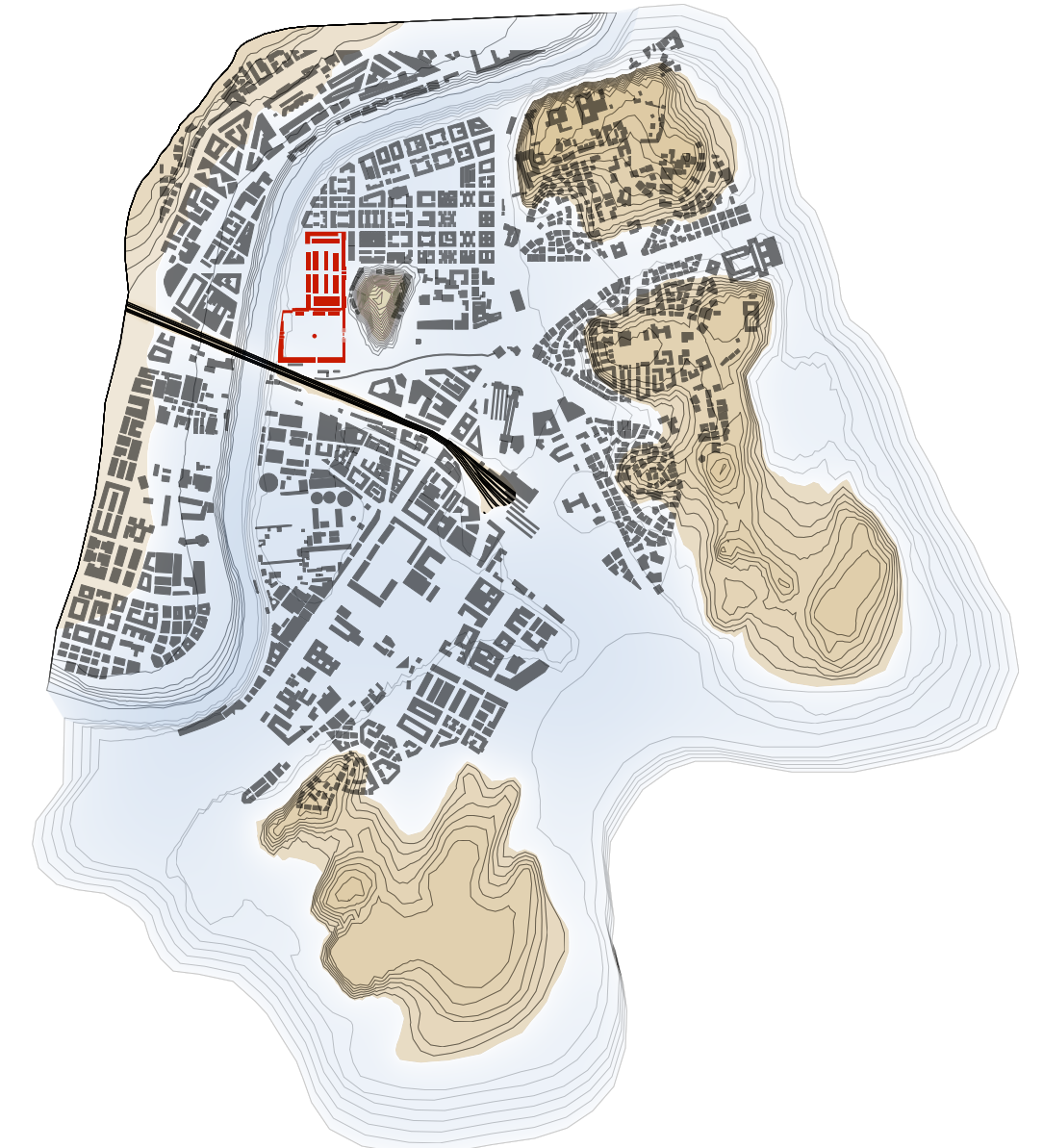
Figure171: Testaccio Vicinity map showing the water level during a flooding event at a water level of 19 meters above sea level
