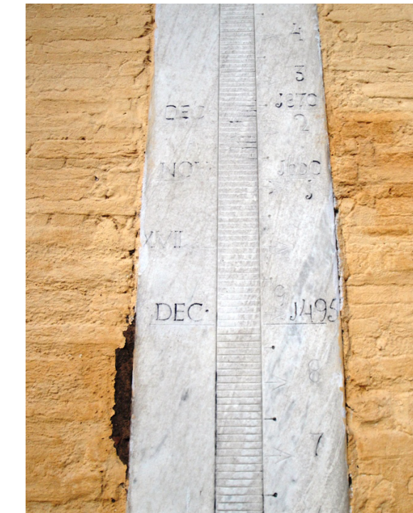
Figure36: Idrometro: On the facade of the Church of San Rocco Church [detail].
