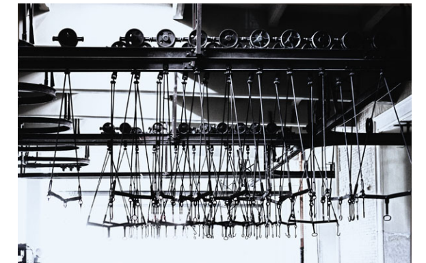
Figure100: Overhead rail system used to transport slaughtered livestock carcasses from one building to another in the Mattatoio.
