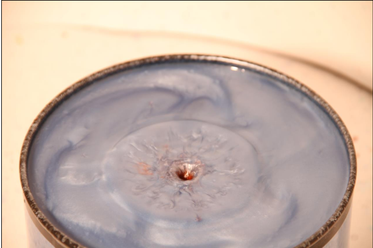
Figure 50. The red droplet follows the blue tower back into the catchment liquid, leaving a small indent from its secondary impact.
