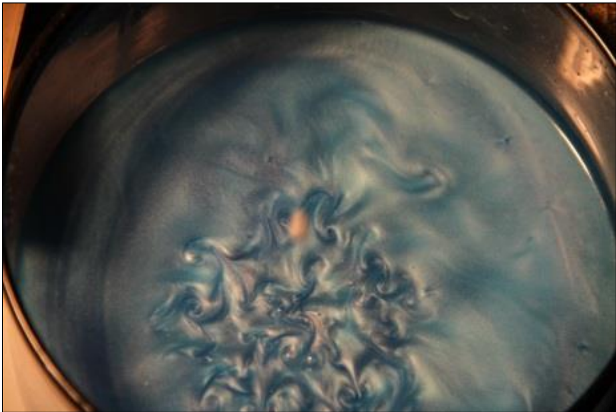
Figure 44. “Old” surface eddies, persisting through the multi-second delay between droplet impacts. In fact, the surface eddies grow with each additional impact.
