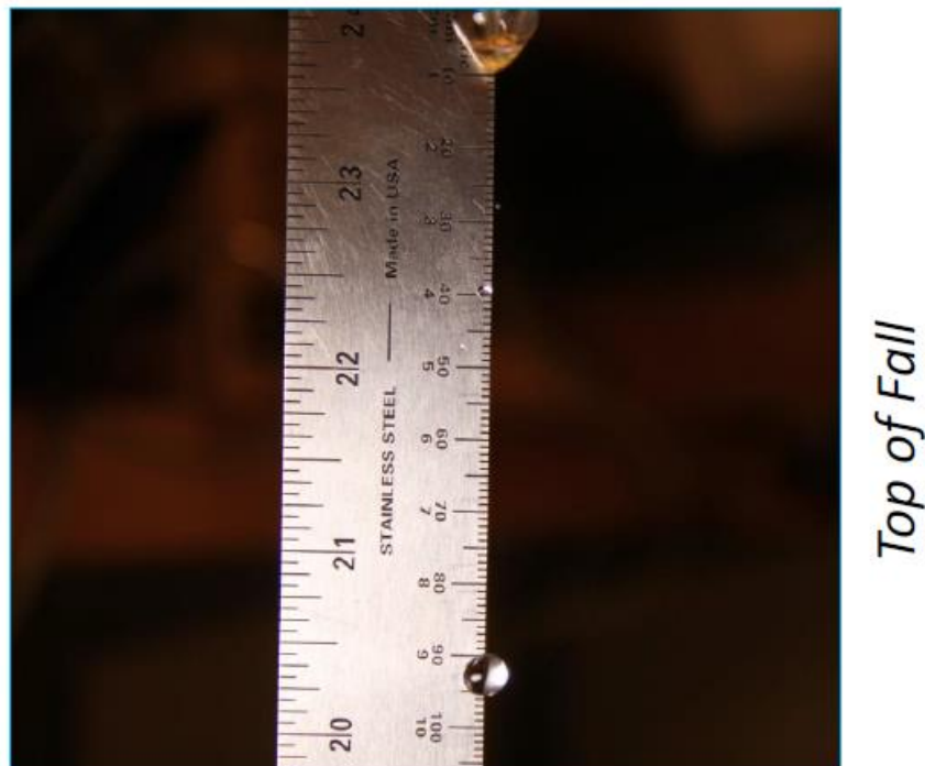
Figure 29. A droplets falling through the first few centimeters of their trajectory. Note the less-than-perfect spheroid shapes. These droplets were still oscillating from their initial release. The dropper nozzle can be seen at the top of the image.
