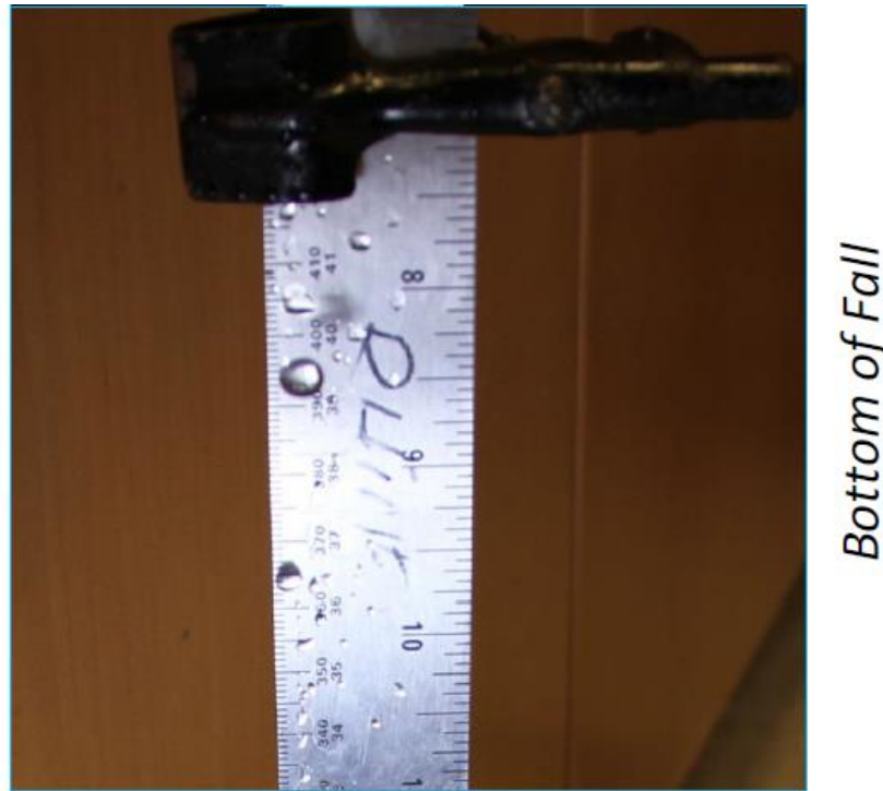
Figure 30. A droplet falling through the last few centimeters of their trajectory. Again, note the less-than-perfect spheroid shape of the droplet. Even towards the bottom of its trajectory, the droplet is still oscillating from the release.
