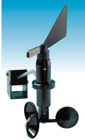
Figure 5. Built by Walker Marine Instruments, the model 2050 Mk 2 is considered a low-end weather station for use atop the mast of small yachts. The retailers, Lilley and Gillie, indicate the anemometer has an accuracy of \pm 0.5 knots with 0.1 knot resolution, and the vane is accurate to within \pm 3 degrees with 0.1 degree of resolution. [13]
