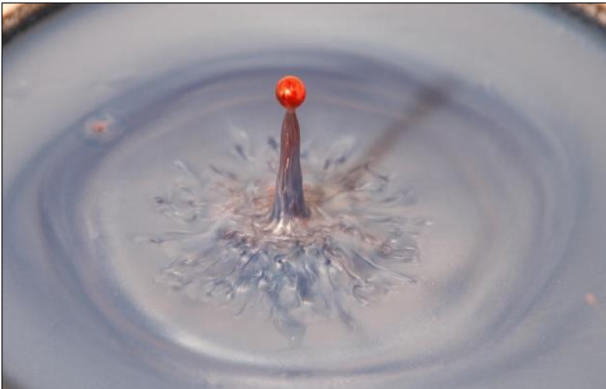
Figure 38. The fourth rheoscopic fluid droplet experiment, allowing for clear visualization of impact splash composition and impact shear stresses.
