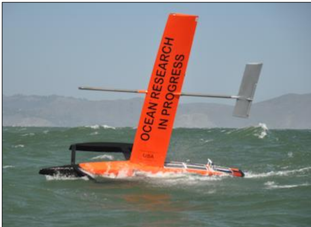
Figure 74. The SailDrone prototype recently sailed from San Francisco to Hawaii and back, autonomously.
