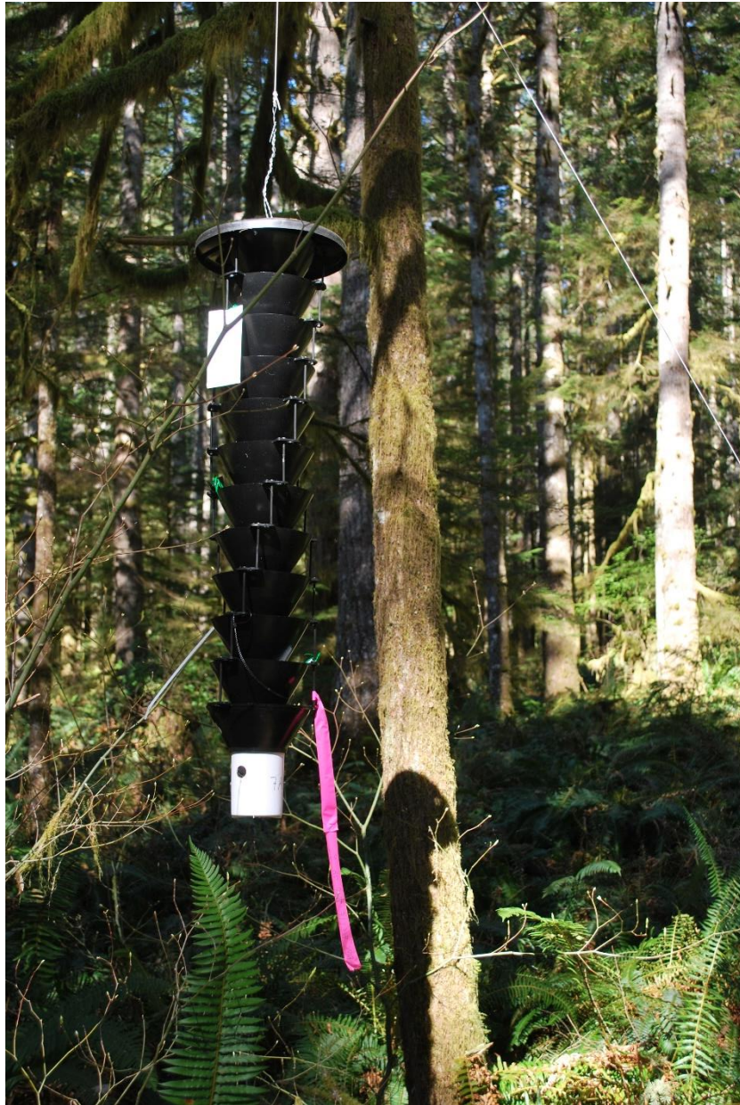
Figure 2.2. Lindgren 12-unit funnel trap used to sample Douglas-fir beetle. Lures include 6-ml low-release packet of ethanol (attached to top funnel), a packet containing 2745 \mu\text{l} of frontalin (1,5-dimethyl-6,8-dioxa-[3,2,1]-bicyclooctane) and 250 \mu\text{l} of seudenol (3-methyl-2-cyclohexen-1-ol) (attached to 6 th funnel from bottom), and a 15 ml packet of Douglas-fir kairomone blend (2 nd from bottom funnel). At the bottom of the funnels in a collection container (white) filled with propylene glycol, a nontoxic antifreeze.
