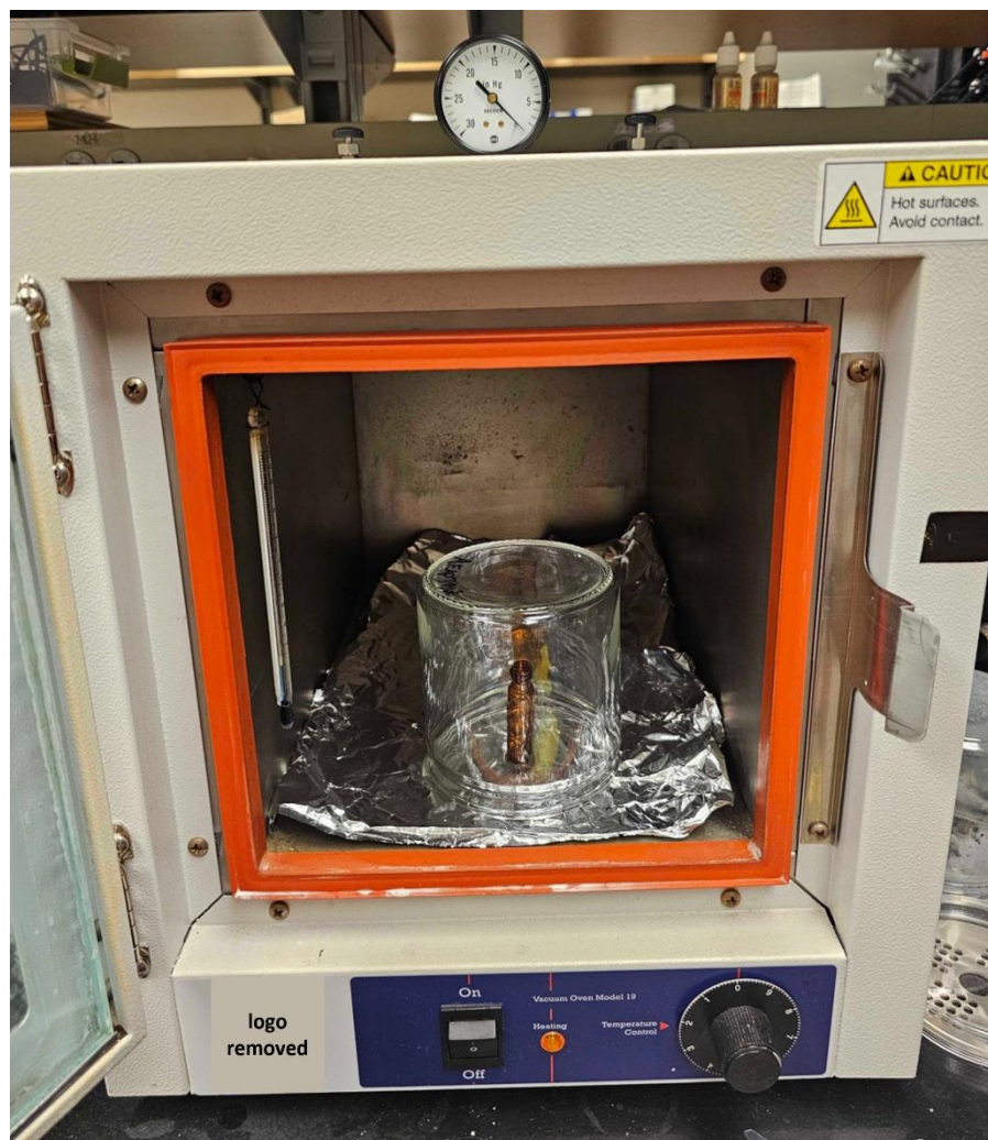
Figure S26. The experimental setup used for amino-silane vapor treatment.
