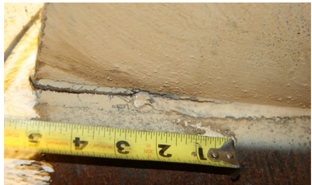
c. 5 in. (bottom) & 2.5 in. (top) weld crack at -1.8% drift
