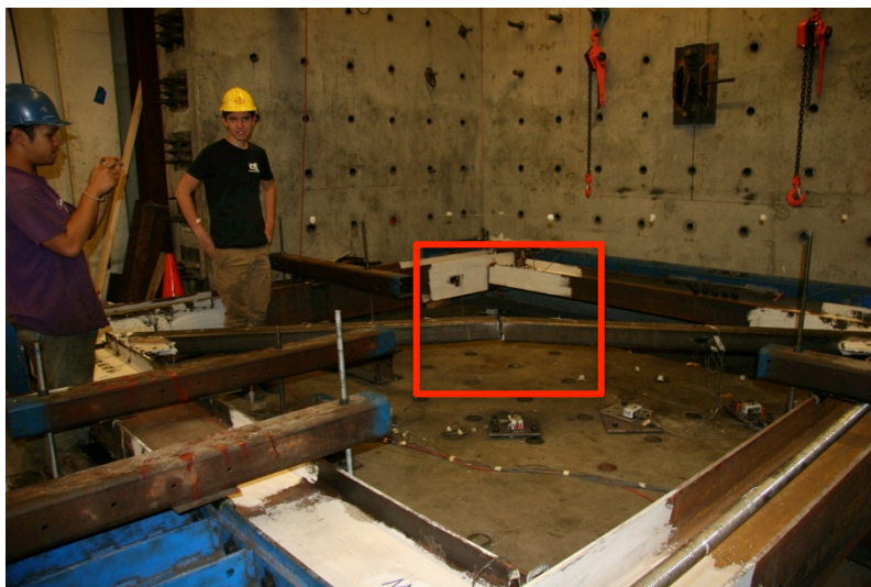
Figure 5.21 - Brace Fracture (BF) at +2.2% Drift
