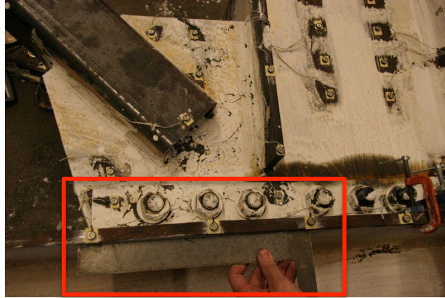
Figure 5.13 - NE Corner Local Flange Buckling (B1) at -1.0% Drift
