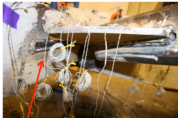
b. OOP Rotation of North Gusset Plate
