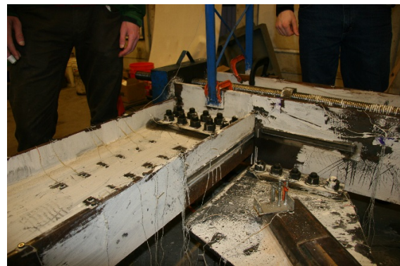
b. Weld Fracture, WBF
