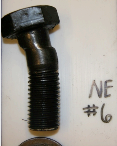
b. Bolt Deformation, BD
