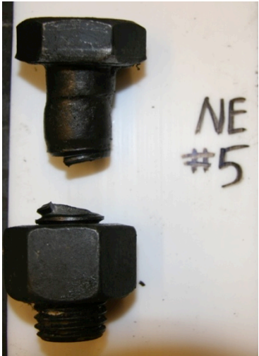
c. Bolt Fracture, BoF
