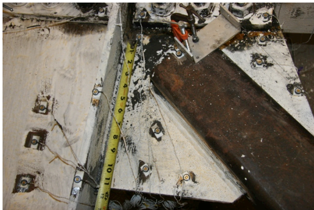
c. 11.25 in. (bottom) & 11.25 in. (top) weld crack at -1.6% drift
