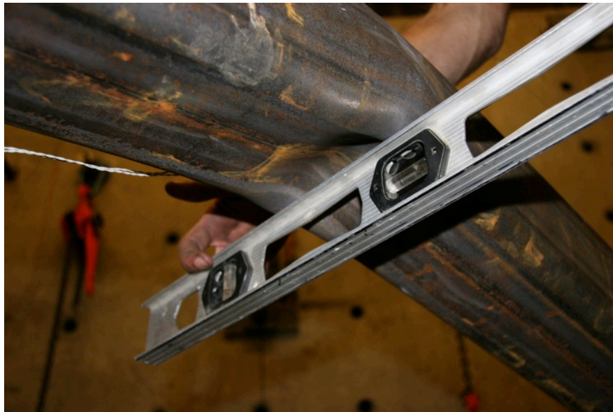
Figure 5.18 - Brace Local Deformation (B3-Cupping) at Midspan at -2.7% Drift
