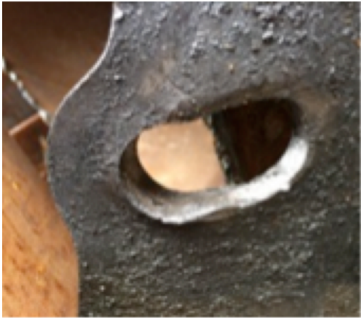
a. Bolt Hole Elongation, BoE (shown in GP)
