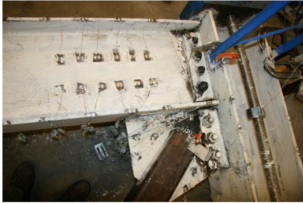
d. Weld fracture at +0.88% drift
