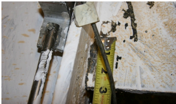
c. 5 in. (bottom) & 2.5 in. (top) weld crack at -1.8% drift
