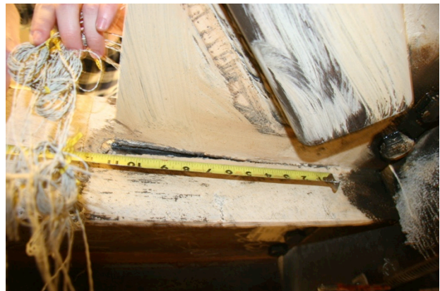
c. 11.25 in. (bottom) & 11.25 in. (top) weld crack at -1.6% drift
