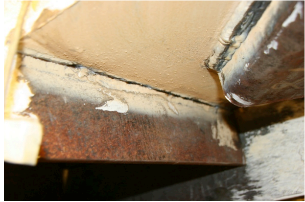
e. Weld fracture at -2.1% drift (second cycle)
