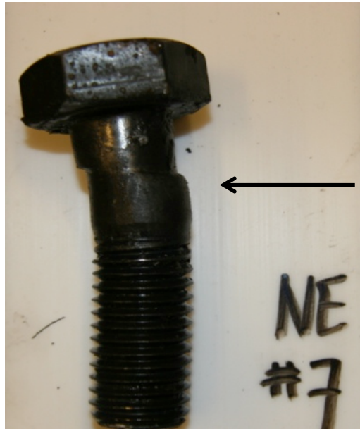
b. Bolt Deformation from NHSS-B3
