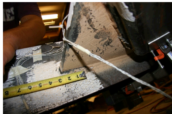
b. 2.125 in. weld crack at -1.9% drift
