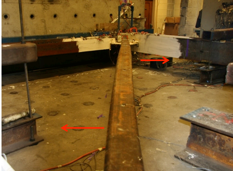
Figure 5.47 - Brace "S" Shape at +1.0% Drift
