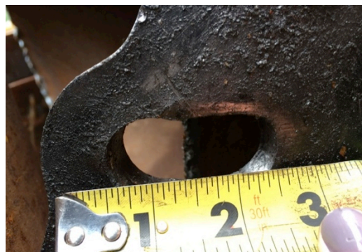
b. Bolt Bearing Deformation from NHSS-B3
