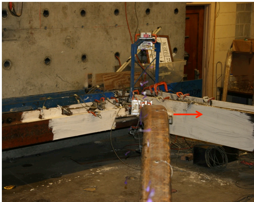
Figure 5.49 - In-plane Brace Buckling at -3.1% Drift
