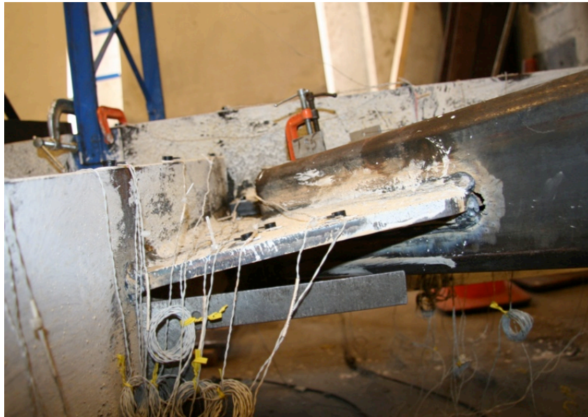
Figure 5.43 - Gusset Plate Rotation at -1.3% Drift
