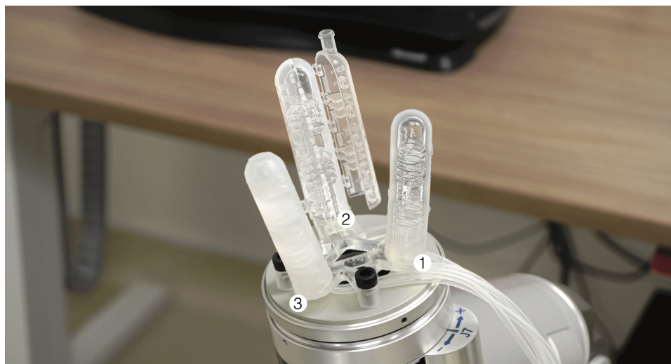
Figure 2.1: Negshell casting used for a three-finger soft robotic gripper. Pictured are three stages of negshell casting from the rightmost to the leftmost finger: 1. 3D-printed structural and negshell cores, 2. The cores placed in 3D-printed molds to be injected with silicone rubber, and 3. A completed finger ready to be actuated.
