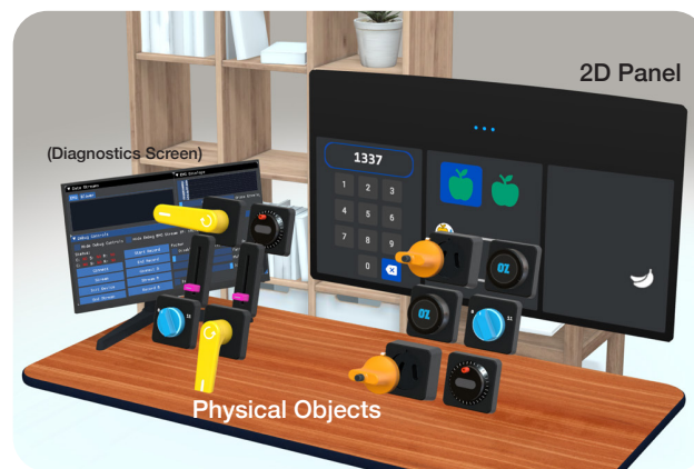
Figure 6.13: A screenshot from within the virtual environment is shown. The physical objects in the foreground can be interacted with like their appearance suggests, such as a knob requiring a twist or a slider requiring a slide. The 2D panel resembles cursor-based or touch-based input similar to modern user interfaces found in VR, computers and smartphones. The monitor is used for diagnostics and is not interacted with during the user study.
