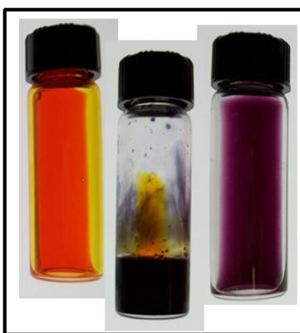
Figure 6.3: Soluble P3HT in xylene (Left), gelled P3HT in xylene (Center), and a suspension of P3HT gel particles (Right).
