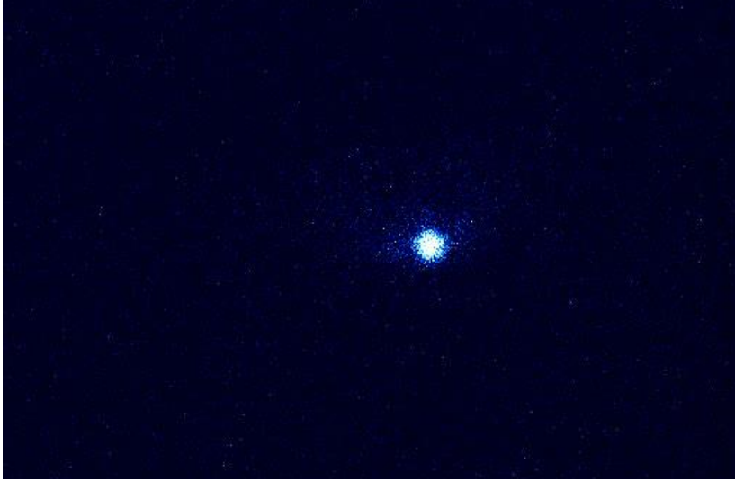
Figure 4.2: A photograph taken from our EMCCD camera of the collected fluorescence from a single trapped barium ion in our ion trap.
