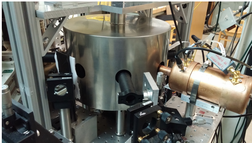
Figure 5.15: Photographs of our magnetic shielding before being installed and in situ .
