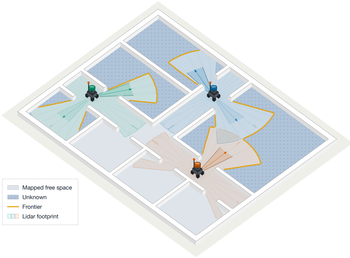
Figure 2.3: Multi-robot exploration . Three robots explore the same environment: the light floor is the space the team has mapped, the dotted region is still unknown, the orange arcs are the frontiers , and the tinted wedges are each robot’s lidar footprint, with arrows marking the frontier it is heading for. The view is an external one, the sum of everything the team knows, but which no single robot possesses.
