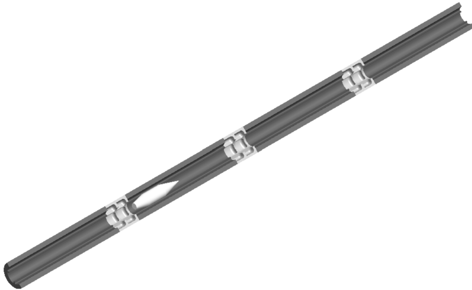
FIGURE 2.20: Schematic of a proposed rail sweeper design [45].
