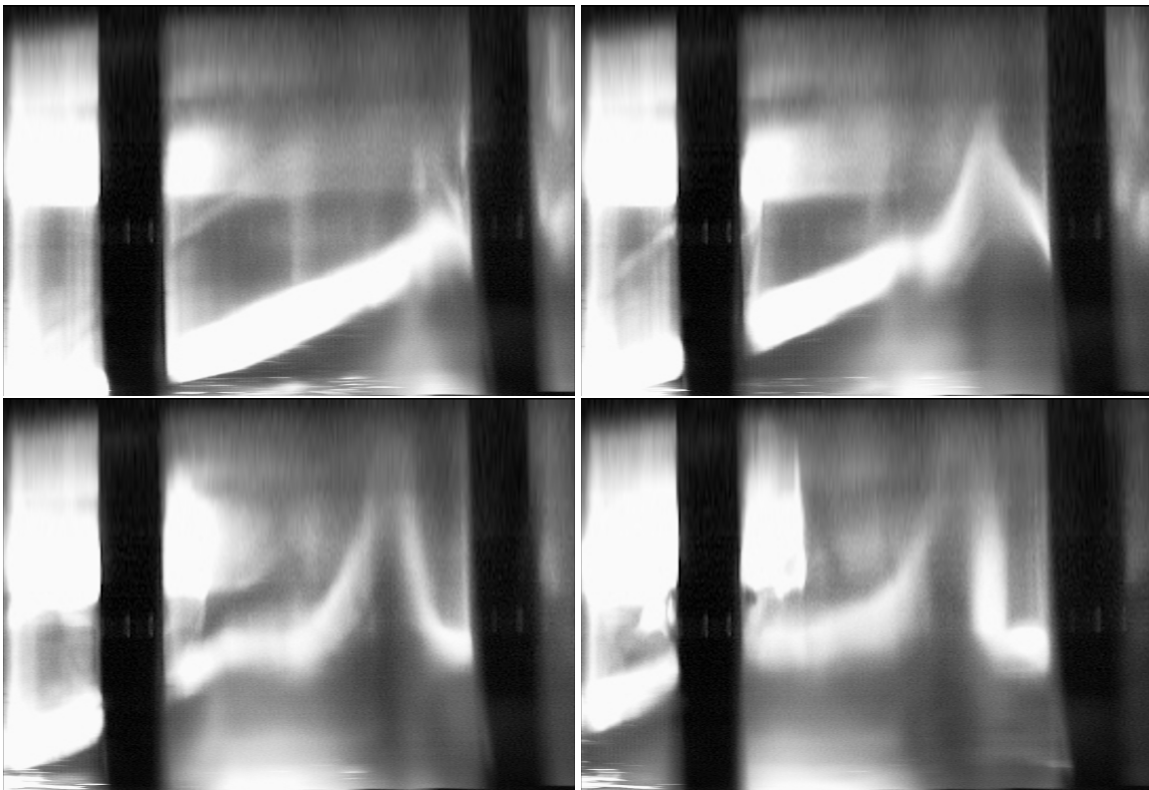
FIGURE 4.9: A 1.496" diameter projectile traveling at Mach 3.42 with 1.5" spacing between baffles.
