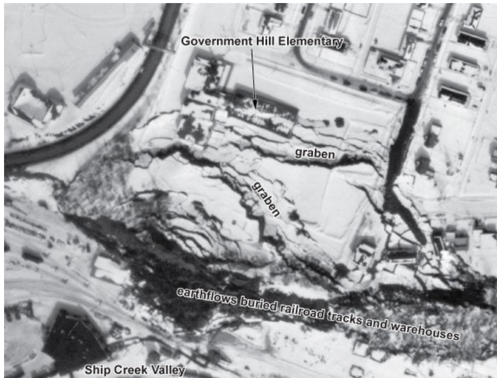
Figure 2.3: Aerial view of the Government Hill landslide in Anchorage, Alaska; occurred during the 1964 Great Alaskan Earthquake (USGS)
