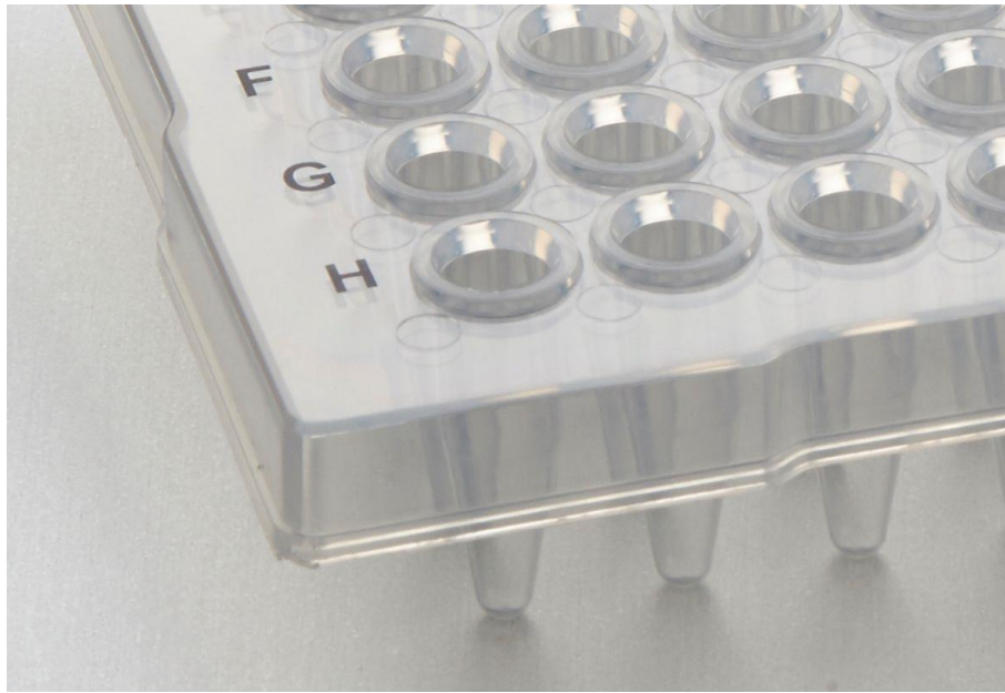
Fig. 2. Closeup picture of 96 well sample plates used in ChIP and with PIXUL highlighting the conical shape of the wells [10].
